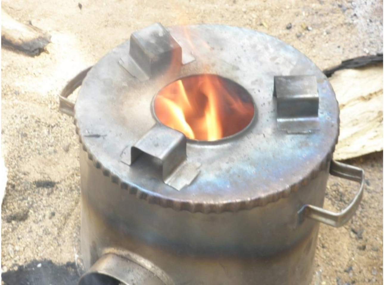
Figure 3.24 Carbonation of the sheet metal above the cone as a result of higher temperature
