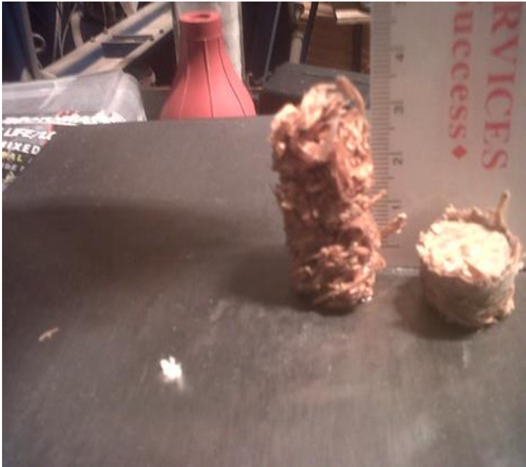
Figure 4.16. Briquettes expanded mostly longitudinally after insertion into water
