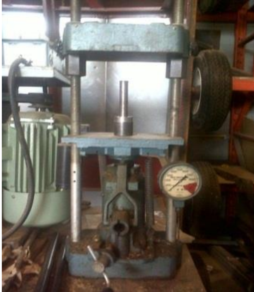
Figure 4.3. Harco manual hydraulic press equipped with pressure gauge
