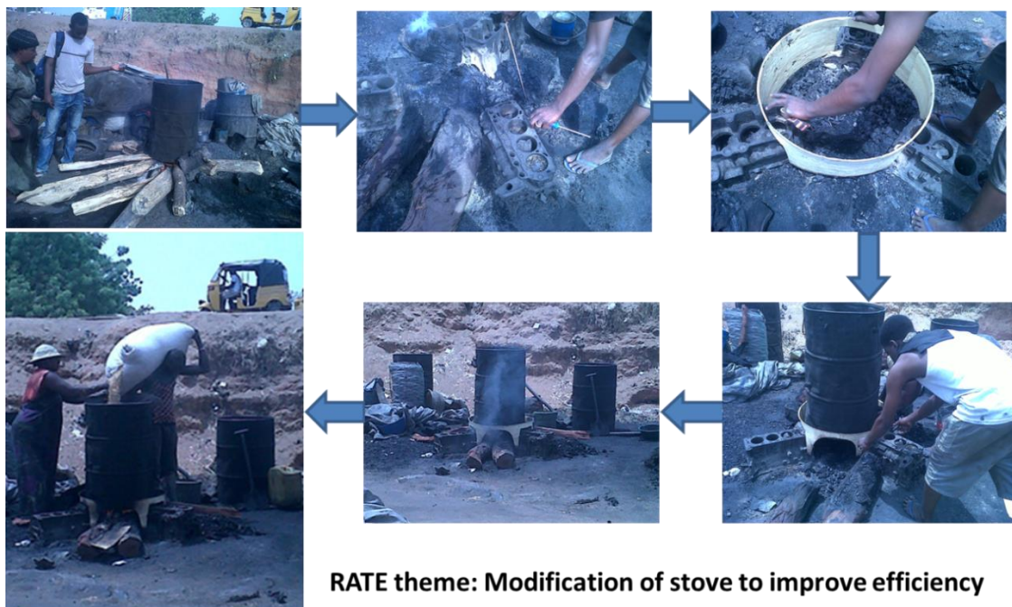
Figure 3.7a. Modification of parboiling stove to improve efficiency using RATE
