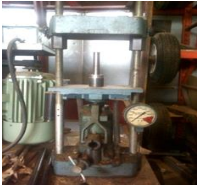
Figure 7.8. Harco manual hydraulic press equipped with pressure gauge
