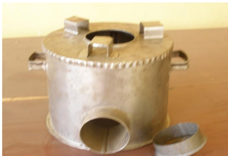
Figure 3.8b. Rice husk stove picture showing the air access port, access port cover, and the flame port
