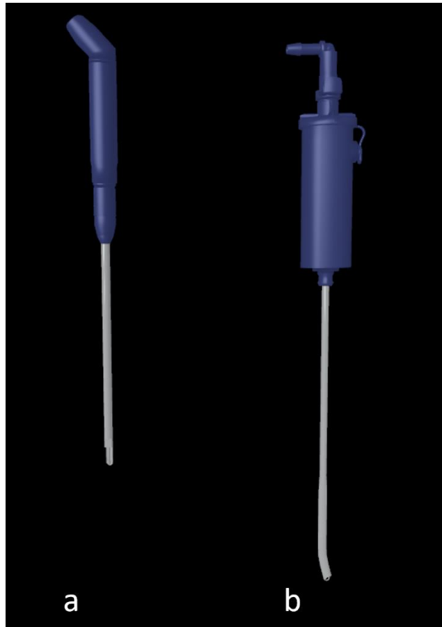
Figure 6.7: Virtual reality (VR) computer-aided design (CAD) models of the a) burr tool and b) Concorde Clear discectomy surgical tools.
