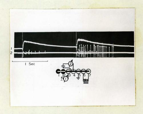
Figure 7. - The responses of a small bundle of muscle fibers to two stimuli in the presence of local veratrine. Channel 1 shows a D.C. record from baths 2 and 3. Channel 2 records the activity of a few fibers with a metal microelectrode in bath 4. 10-7 veratrine sulphate in baths 1 and 2.
