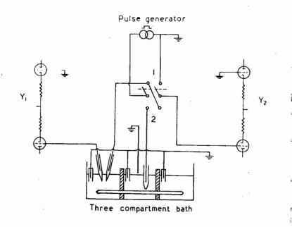
Figure 23. - Arrangement of electrodes for recording the after-discharge at two points along the same fiber. Note: double-pole, double-throw switch; position 1 for testing electrode insertion, position 2 for normal use. Veratrine sulphate put in end compartment containing the proximal end of muscle and the two microelectrodes.
