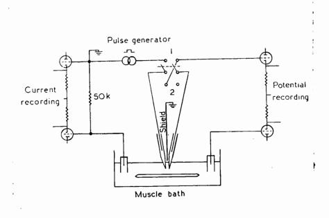
Figure 10. - Arrangement of electrodes for intracellular stimulating and recording. Note the double-pole, double-throw switch, position 2 for inserting stimulating electrode, position 1 for testing electrode insertion and for normal use.
