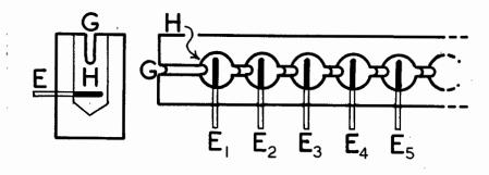
Figure 1. - A diagram of the perspex bath used for mounting strips of the frog's sartorius muscle. For description see text.
