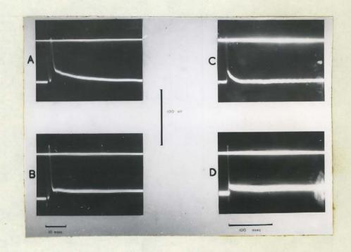
Figure 11. - Responses of single muscle fibers of the frog sartorius recorded with inside-the-cell electrodes. In A and C are two responses from the same fiber when the muscle was immersed in tubocurarine-Ringer solution. In B and D are two responses from the same fiber when the same muscle was immersed in a 10-8 veratrine sulphate solution.
