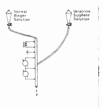
Figure 9. - Perfusion arrangement for obtaining local veratrine application. The lower two recording electrodes were moveable to locate the site of origin of repetitive responses and the potential gradient along the muscle.
