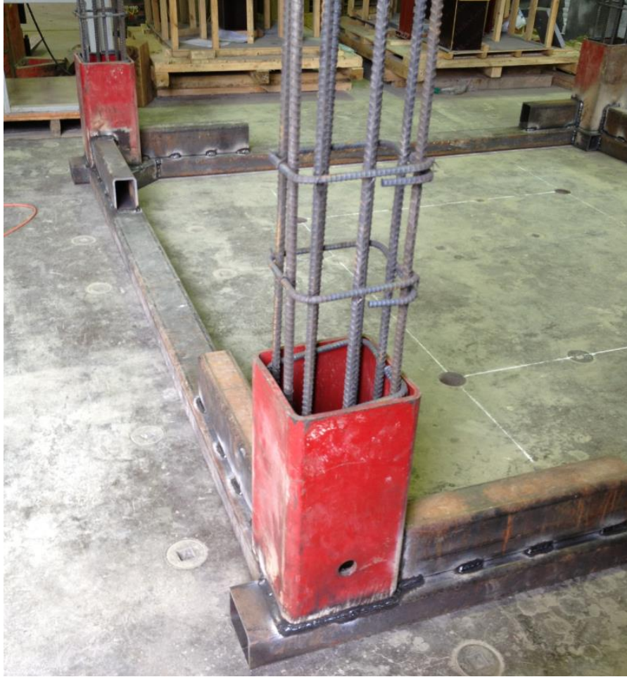
Figure 2-10: (a) Steel frame base; (b) Welding column reinforcement to the steel frame; (c) Welding HSS steel shoes to the steel frame
