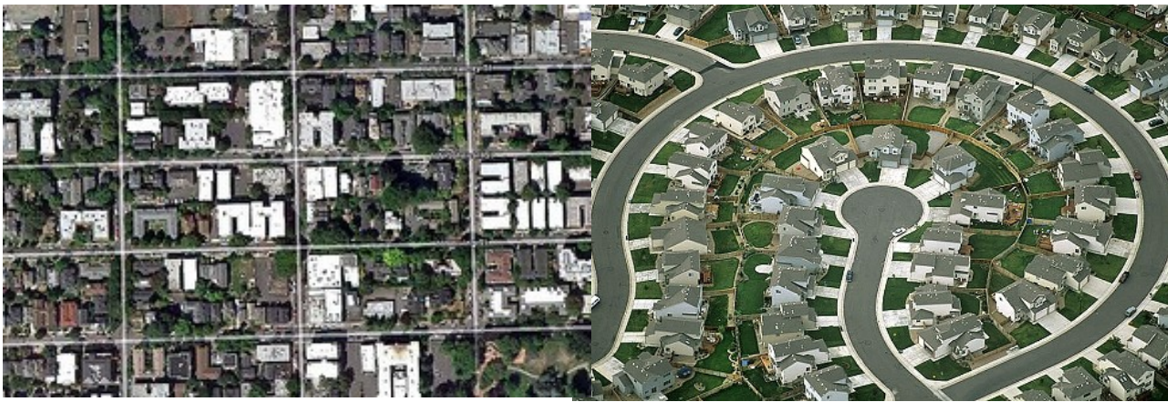
Figure 1.5 High (left image) and low (right image) connectivity neighbourhoods (Images taken from www.switchboard.nrdc.org ; www.google.ca/maps and www.airphoton.com )
