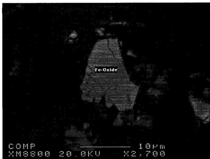
**Figure 4. 31 Electron microprobe analysis of PoT sample weathered in no hole cover showing maghemite**
