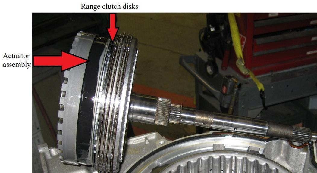
FIGURE 2.1. Range clutch pack with the transaxle
