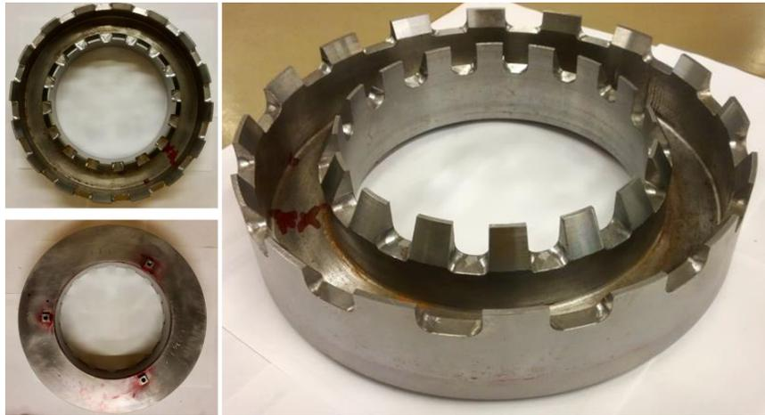
FIGURE 6.16. Machined stator
