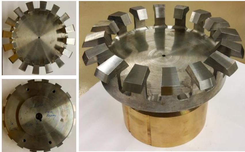
FIGURE 6.15. Machined rotor
