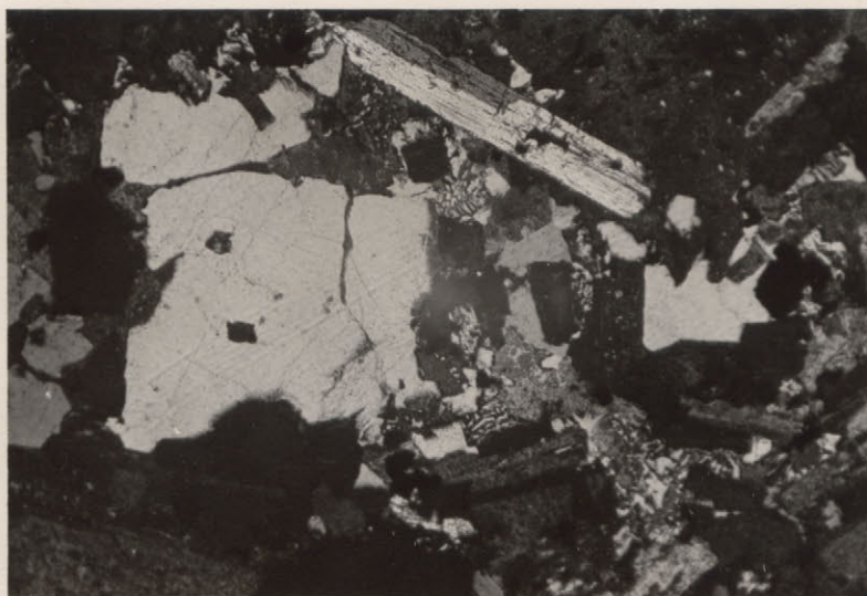
Fig. 8. Specimen No. B209'50. Large irregular grains of albite and a twinned crystal of hornblende are surrounded by interstitial micropegmatite. (Crossed nicols, x 30)
