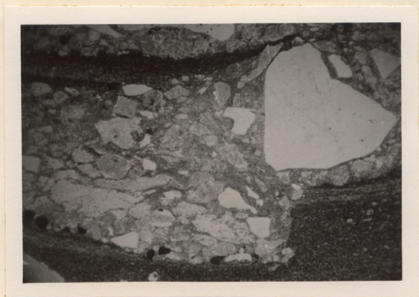
Fig. 16. Specimen No. B24'51. Contact between shale and coarse grit. Channelling in the shale indicates that the top of the beds is towards the top of the page. (Plain light, x 30)
