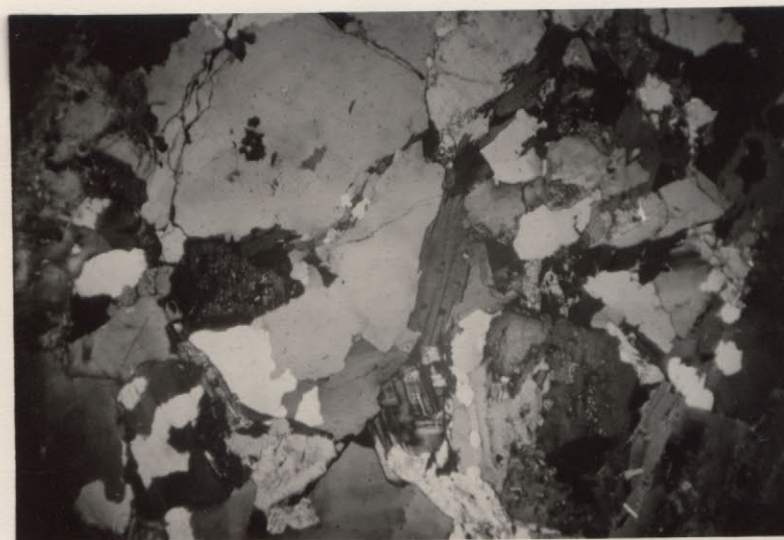
Fig. 9. Specimen No. B177C'51. Boyd's Pond granite showing fractured quartz crystals, biotite with pleochroic haloes, and interstitial microcline. (Crossed nicols, x 30)
