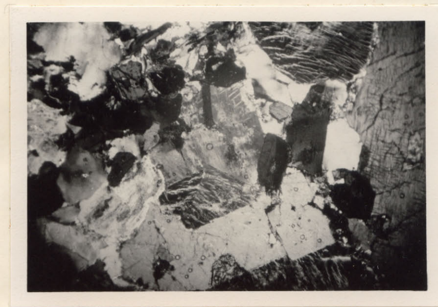
Fig. 10. Specimen No. M15'51. Biotite granite showing the abundance of perthitic feldspar. (Crossed nicols, x 30)
