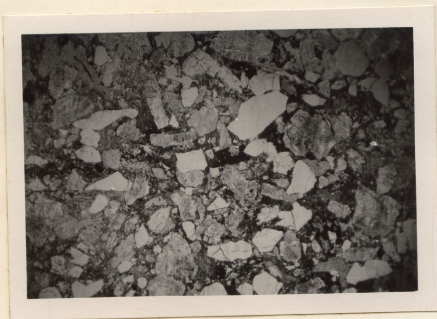
Fig. 15. Specimen No. B72A'50. Volcanic grit showing the angularity of the quartz grains. (Crossed nicols, x 30)
