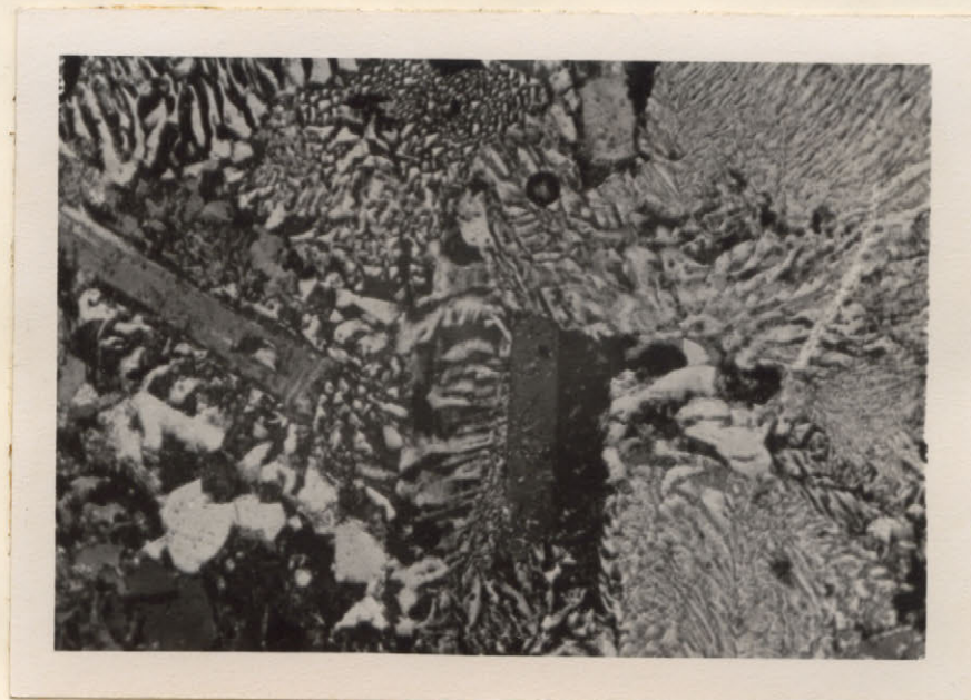
Fig. 11. Specimen No. B195'51. Granophyre dike, showing phenocrysts of albite enclosed by a micropegmatitic intergrowth. (Crossed nicols, x 60)
