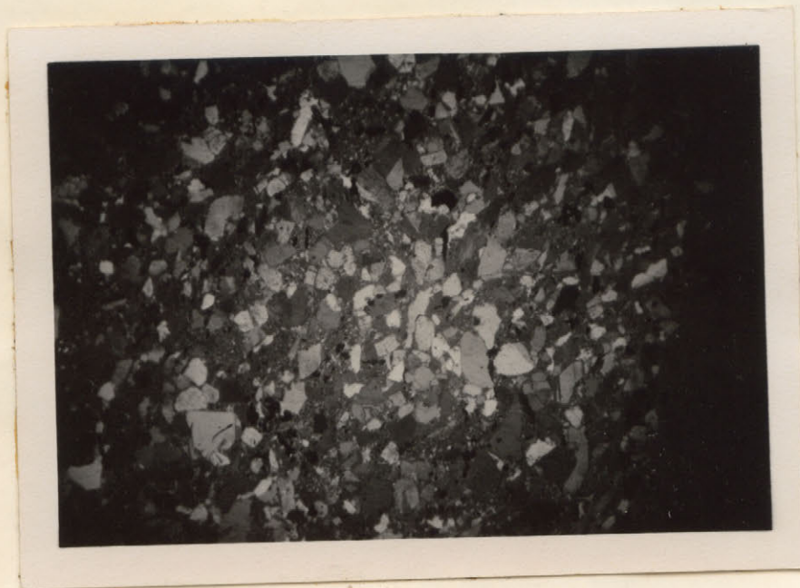
Fig. 14. Specimen No. SS1'51. Sandstone showing a rough parallelism of the long axes of the quartz and feldspar grains. (Crossed nicols, x 30)
