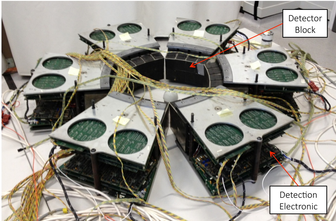
Figure 4.7 – Double ring assembly of ECAT 951 modular detector blocks.
