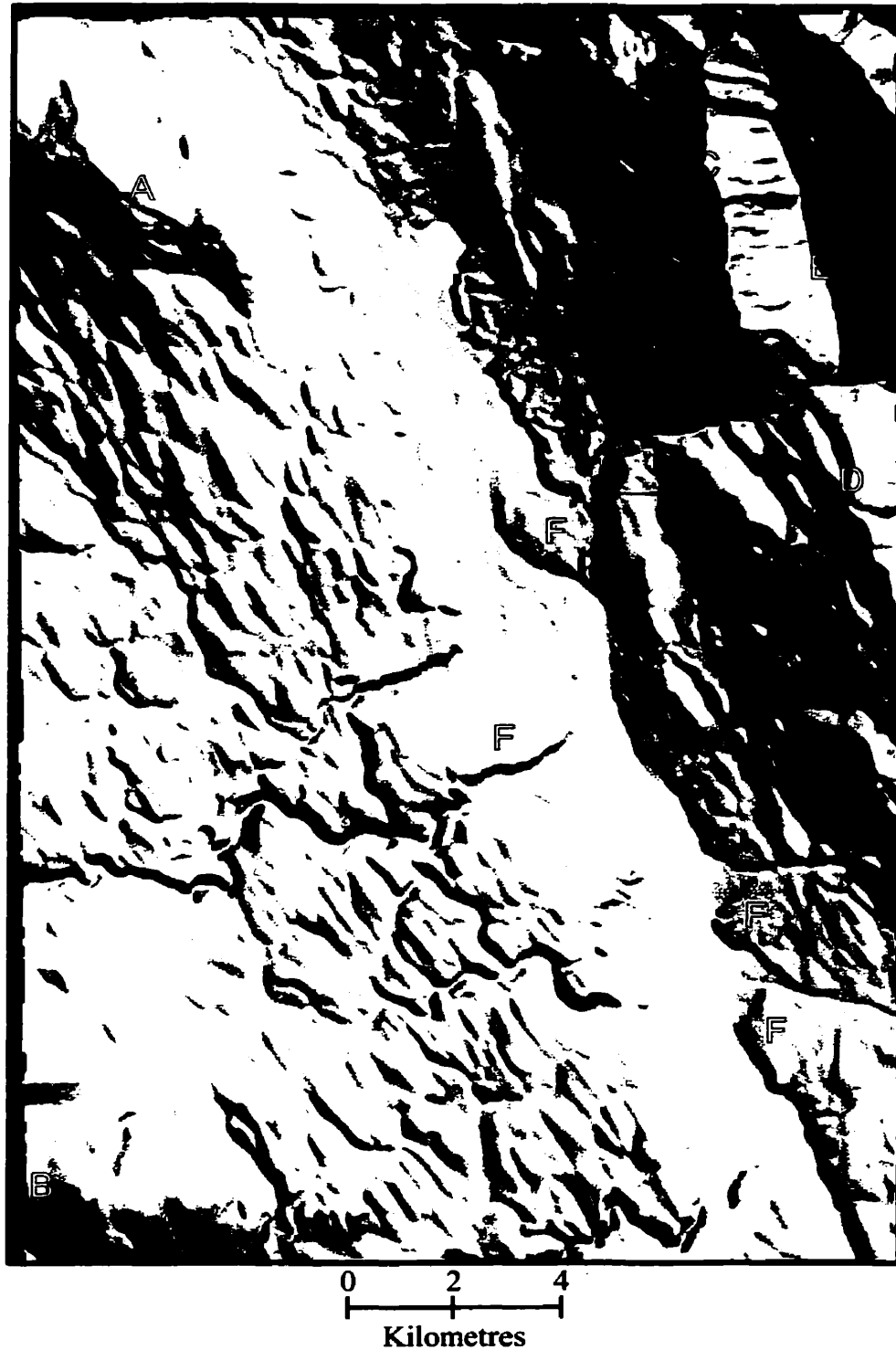
Figure 3.4 Shaded Digital Elevation Model of the study region. The DEM is illuminated from the northeast and has been smoothed with a 3 X 3 mean filter. A=Steamboat Mountains, B=Mount Bruce, C=Mount Berland (Brisco Range), D=Redstreak Mountain (Stanford Range), E=McKay Creek, F=benches. The outlines of Kootenay National Park and Dry Gulch Provincial Park are shown in grey.
