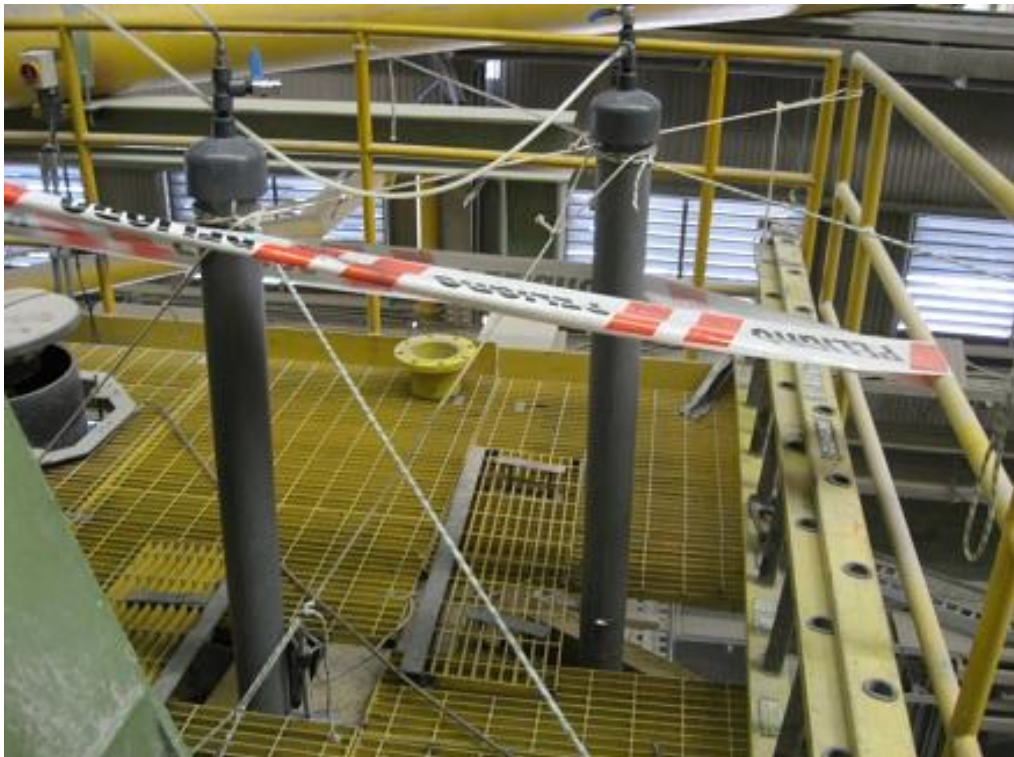
Figure 6. 16 Picture of the J_g sensor installation at Chuquicamata concentrator: J_{g1} , J_{g2} and J_{g3} (above); J_{g4} and J_{g5} (below)
