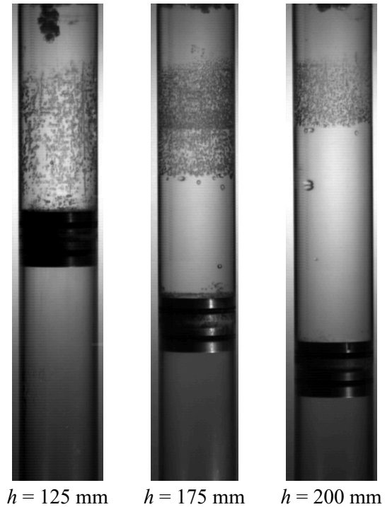
FIG. 15. Images of cavitation onset for typical experiments at different heights (Multimedia available online). The experimental conditions are: (left) h = 125 \text{ mm} , p_{t,max} = 4.0 \text{ MPa} , and v_{p,max} = 10.1 \text{ m/s} , (middle) h = 175 \text{ mm} , p_{t,max} = 3.7 \text{ MPa} , and v_{p,max} = 8.89 \text{ m/s} , (right) h = 200 \text{ mm} , p_{t,max} = 4.0 \text{ MPa} , and v_{p,max} = 10.4 \text{ m/s} .
