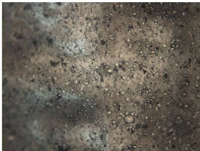
**Figure 4.12** Optical microscopy image of sc-CO<sub>2</sub> film embedded with caffeine (no visible crystals).
