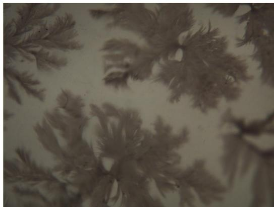
**Figure 4.10** Optical microscopy at 40X of caffeine crystals on the surface of a press dried film.
