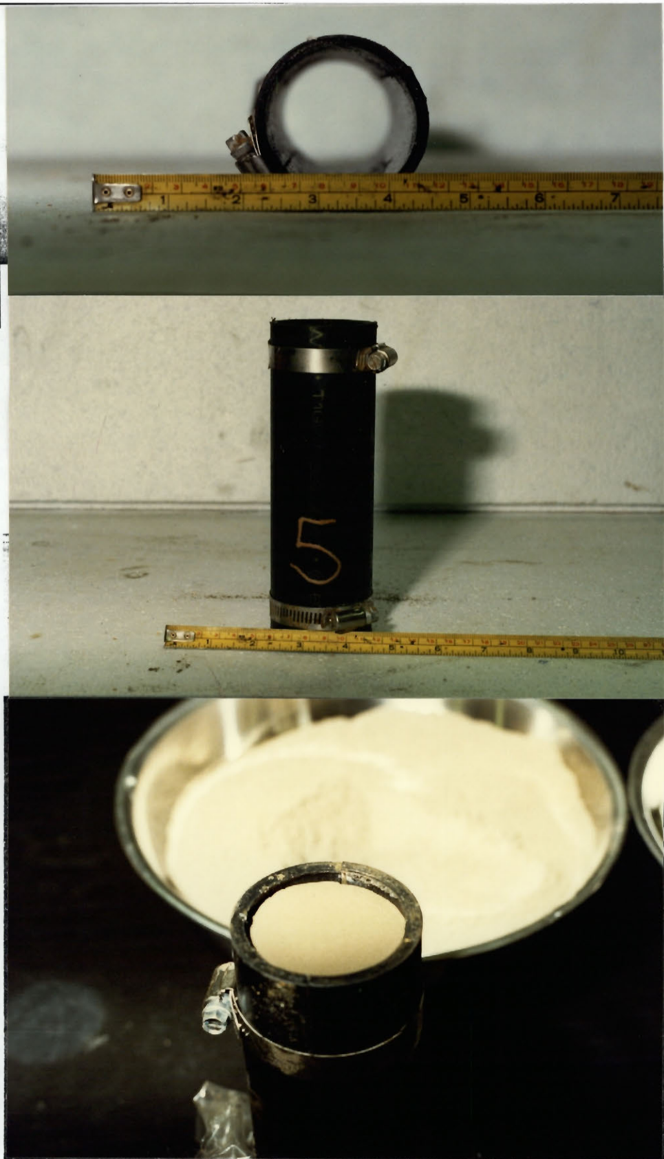
PLATE 2: CYLINDRICAL SPECIMEN MOLDS WITH INTERNAL DIAMETER OF 50 mm AND LENGTH OF 130 mm.
