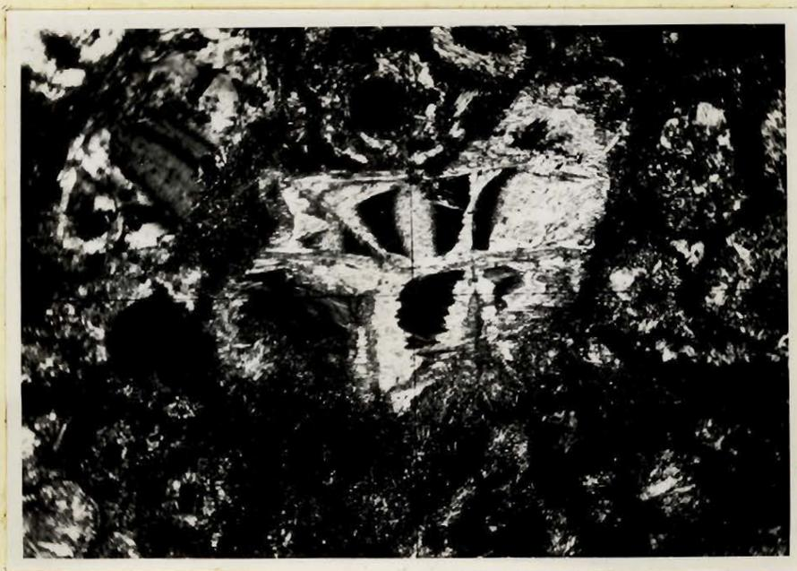
Figure 1. Talc ( white ) replacing serpentine ( dark ).
