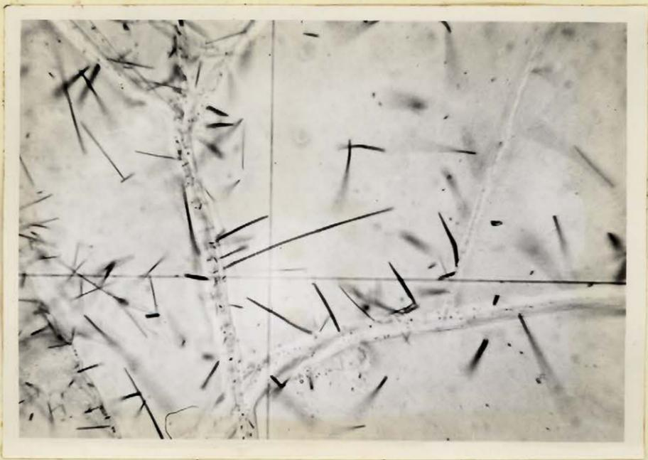
Figure 2. Rutile needles in serpentine. Ordinary light.
