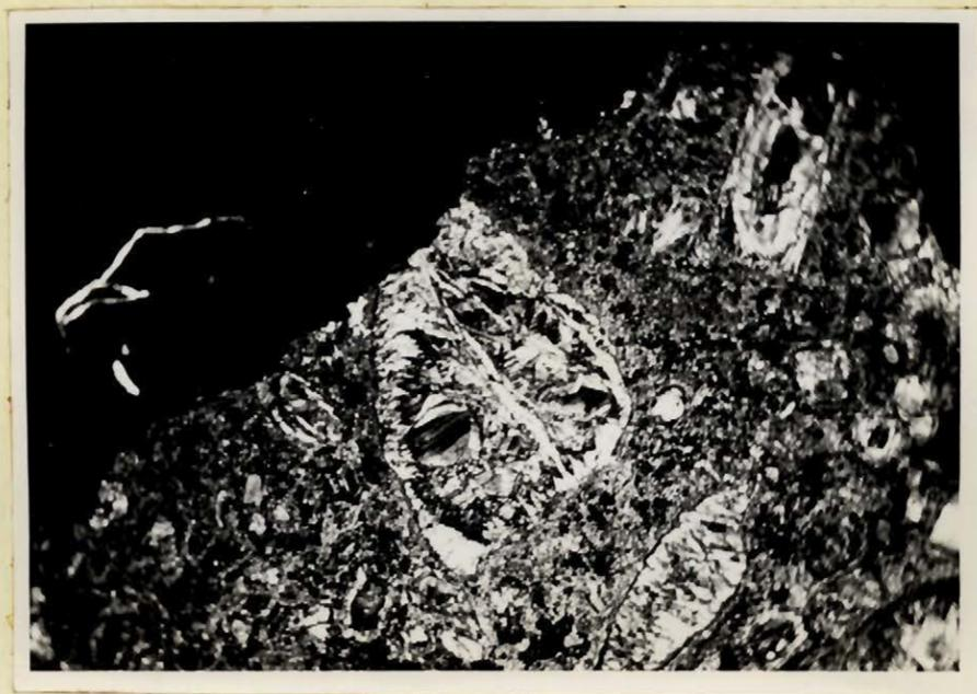
Figure 2. Serpentine with "mesh" structure. Crossed nicols.
