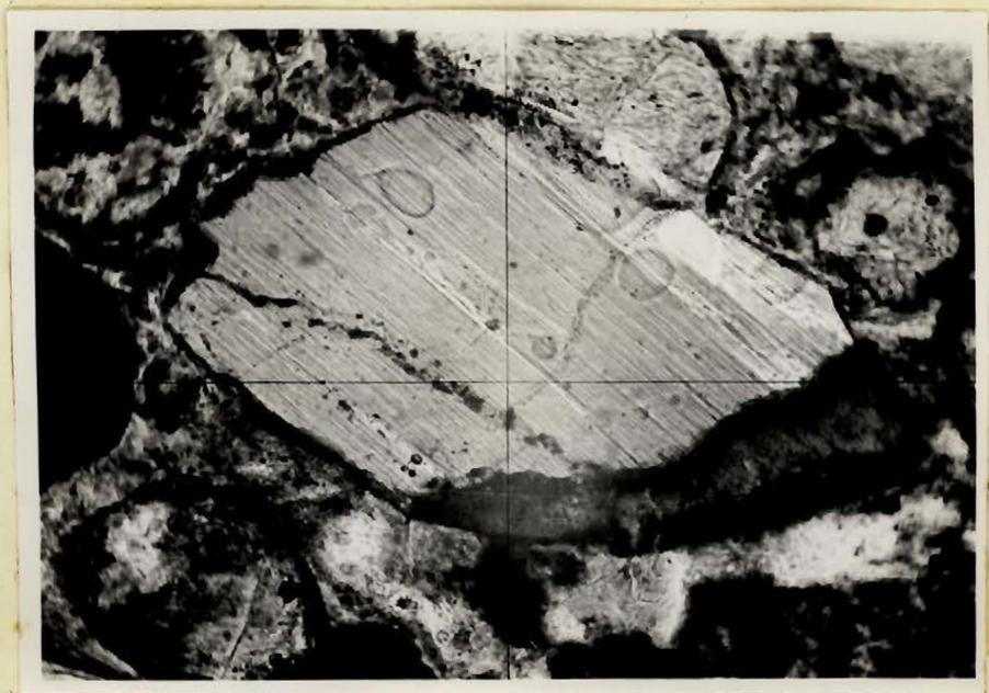
Figure 2. Hypersthene, showing reaction rim. Ordinary
