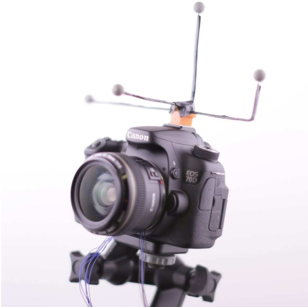
Figure 1–2: The camera and one of the modified lenses we use for recording videos with automatic focus pull using predictive filtering. Blue wires attached to the lens allow direct control of the lens from a computer using a serial communication protocol. Four small retro-reflective markers mounted on top of the camera allow its position and orientation to be tracked with a motion capture system.
