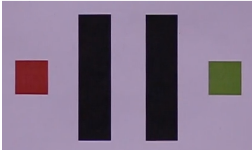
Figure 5–2: Our custom focus target with sharp white to black edges used to measure the blur in each frame of our focus test videos.
