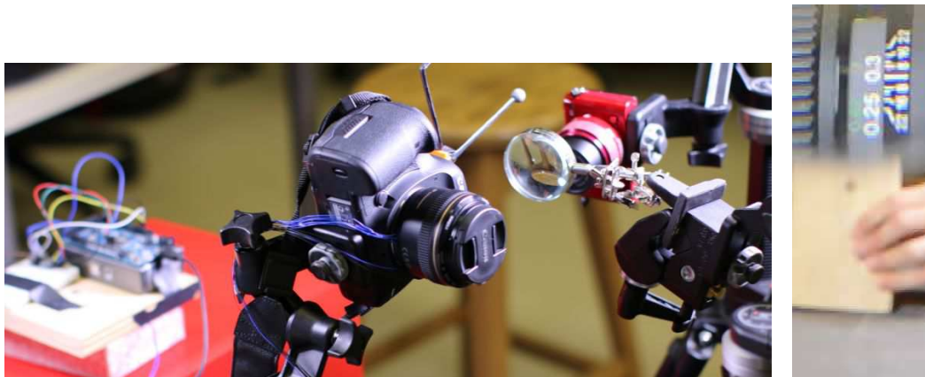
Figure 3–4: Setup for measuring the latency of the system. Left, the configuration of the lens and high-speed camera. Right, the actual view from the high-speed camera, seeing both the lens and the block hitting the table.
