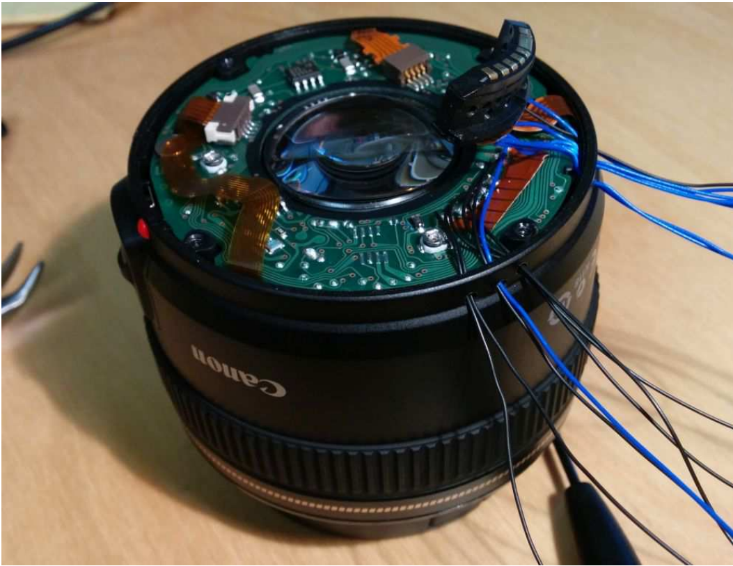
Figure 3–1: Canon EF lens modification, bypassing the connection between the lens and the camera inside the lens.
