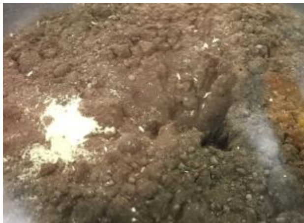
Figure 2.7. Elemental sulphur build up after 10 weathering cycles
