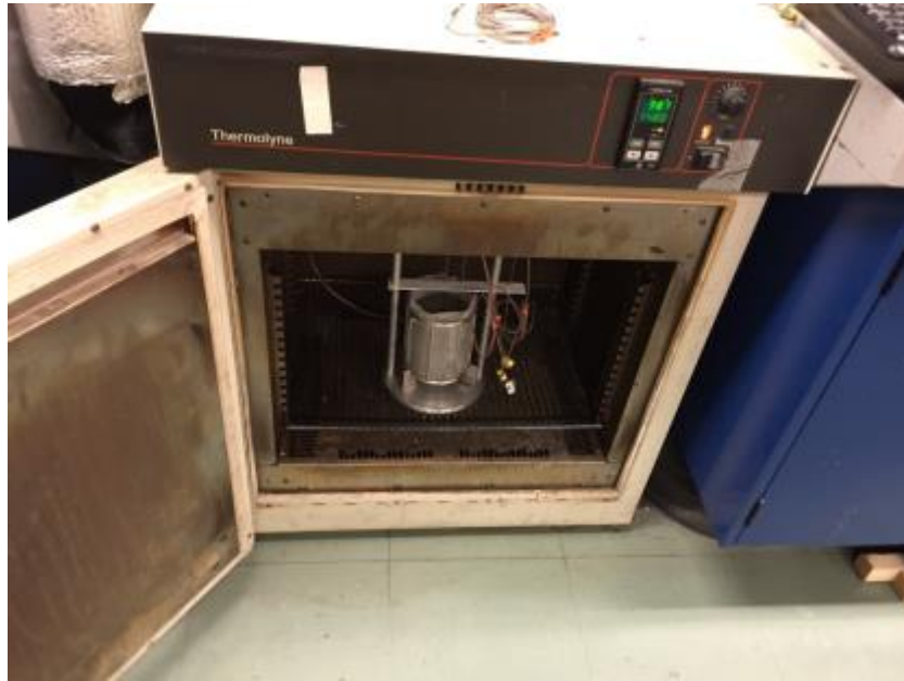
Figure 2.3. U.N. Recommended Test Apparatus in McGill University
