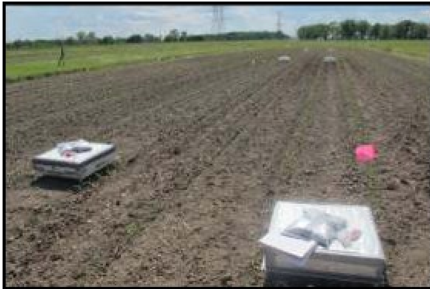
Figure 6 GHGE Sampling Chambers (Hurst, 2012)
