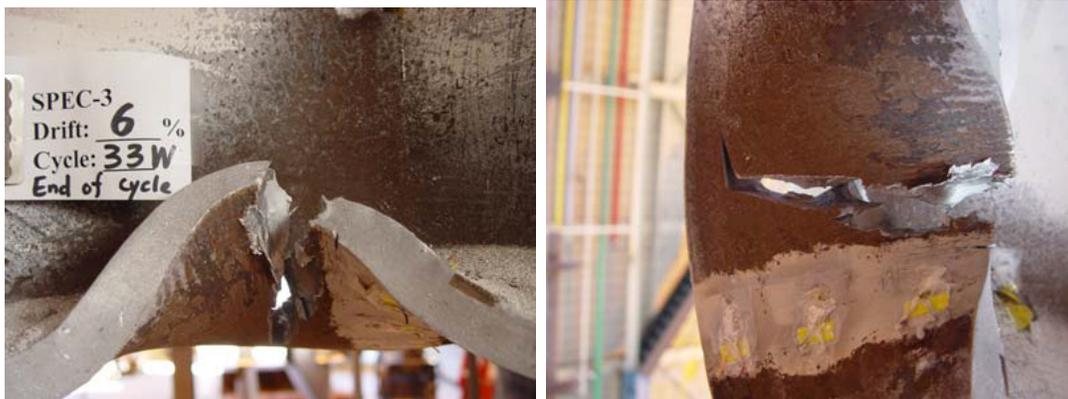
(c) ductile tearing
