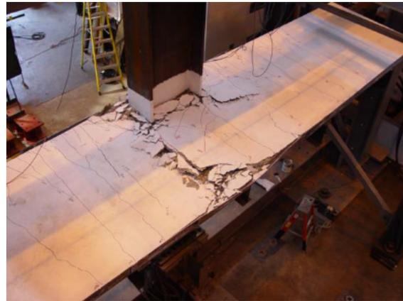
(c) concrete slab cracking and crushing
