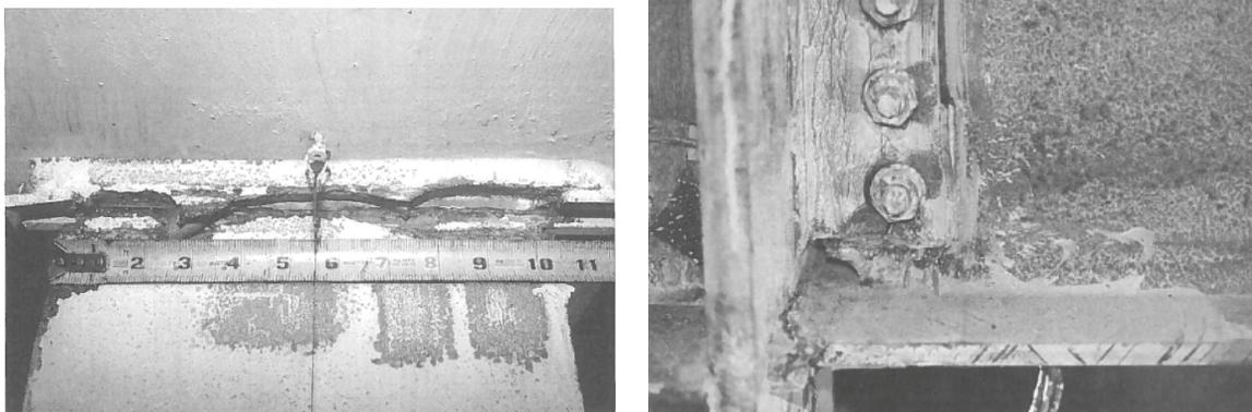
(a) fracture across welded beam top flange
