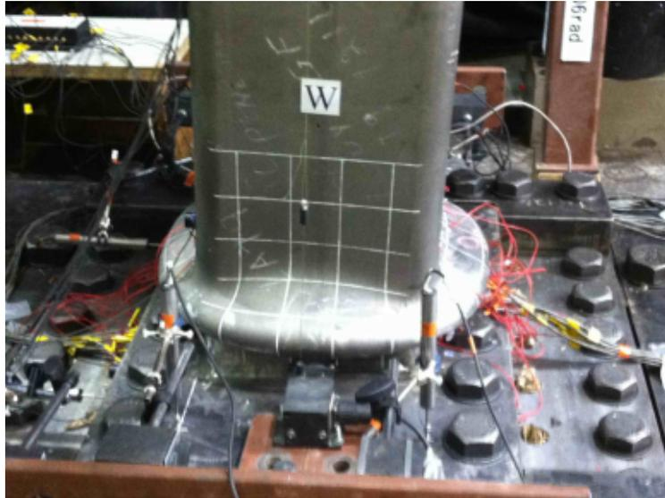
Figure 2.16: Elephant foot local buckling mechanism, from Suzuki and Lignos (2015).
