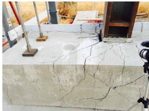
Figure 2.28: Typical failure modes observed in embedded column base connections, from Grilli (2015).
