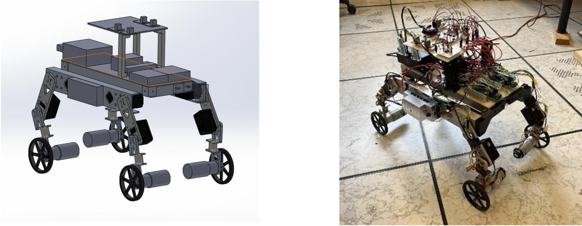
**Figure 3.2:** a) SOLIDWORKS model b) Assembled test platform
