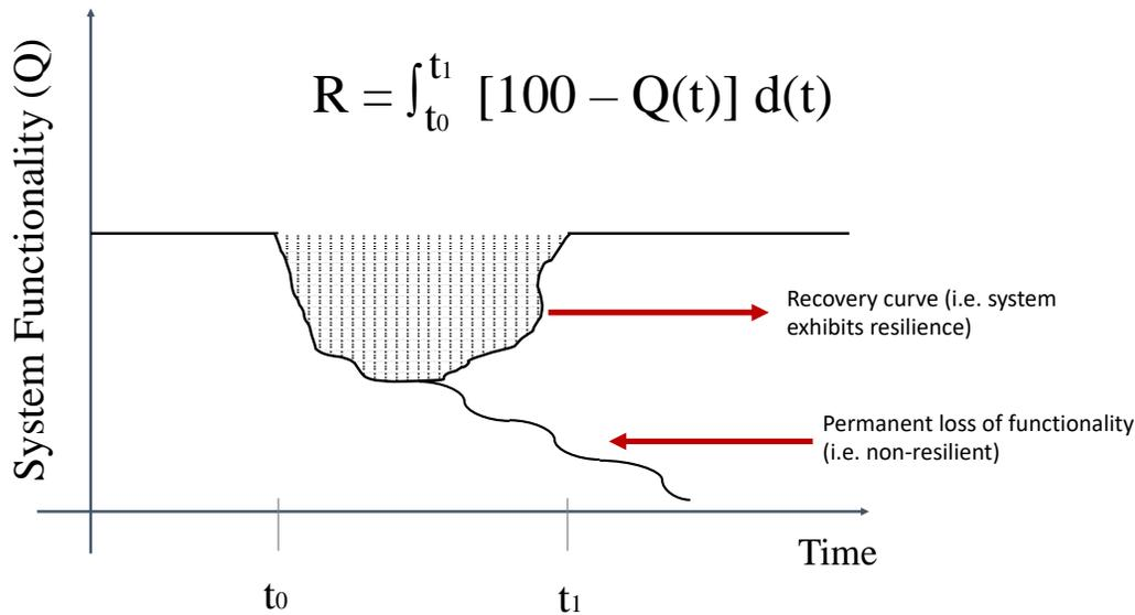
**Fig. 2.3.** System performance before, during, and after disturbance (adapted from *Yodo and Wang, 2016*)
