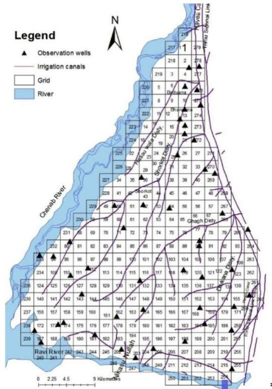
**Fig. 3.2.** Nodal network polygonal configuration of the Rechna Doab watershed with observation wells, canal network, and grid (reproduced with permission: Inam et al., 2017a)
