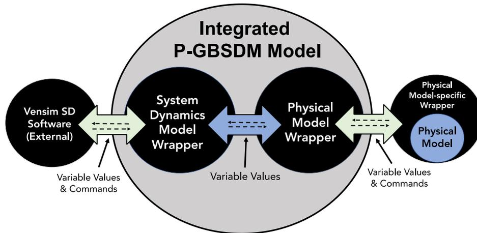
**Fig. 3.3.** Diagram of P-GBSDM coupling using Tinamit as a wrapper (adapted from Malard et al., 2017)
