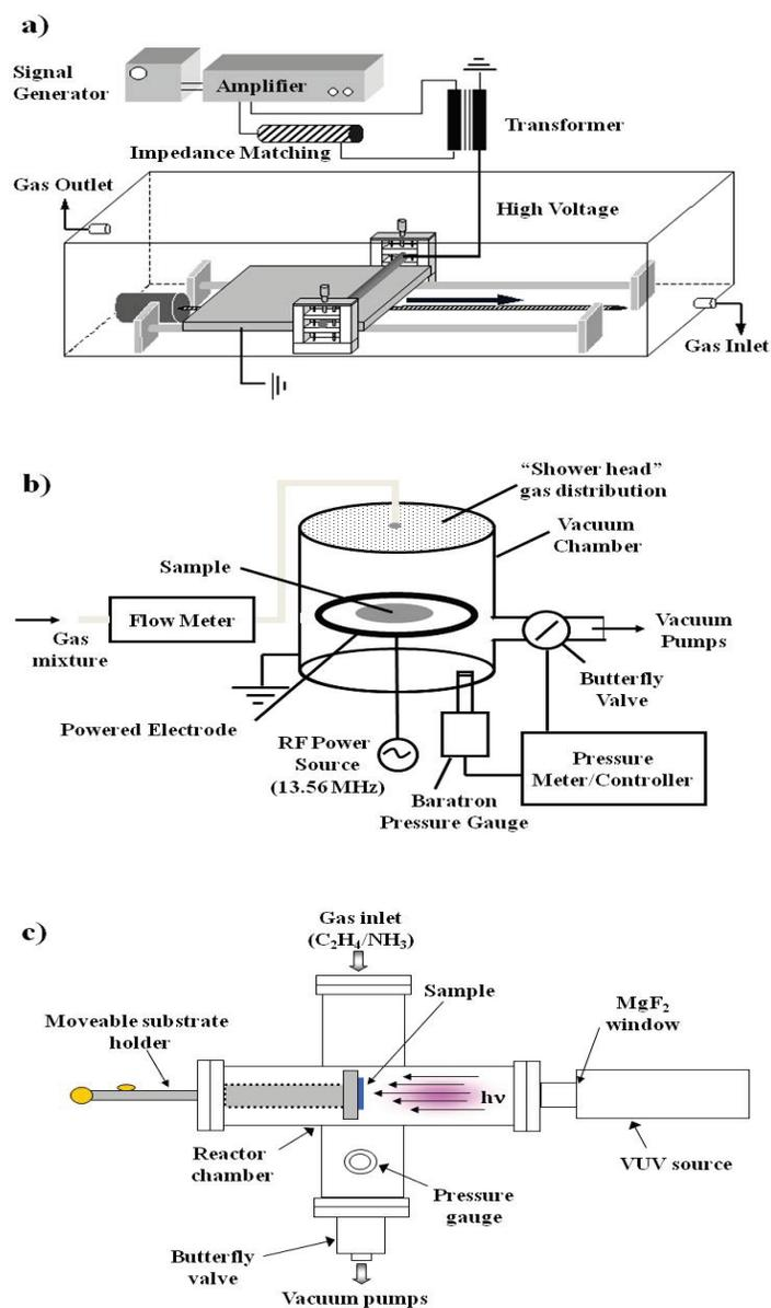
**Figure 1:** Three reactor systems used in the present research: (a) Low-pressure plasma (LP-PECVD), 13.56 MHz r.f. discharge; (b) Atmospheric-pressure dielectric barrier discharge (AP-DBD) plasma; (c) Vacuum ultraviolet photo-polymerisation (VUV-CVD), see text. (From ref. [28], with permission).
