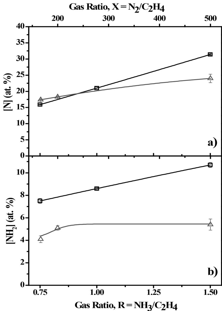
**Figure 2:** (a) Concentrations (in atomic %) of nitrogen,  $[N]$ , and (b) of primary amines,  $[NH_2]$ , in L-PPE:N ( $\square$ ) and H-PPE:N ( $\Delta$ ) deposits, as functions of the gas mixture ratios,  $R \equiv F_{NH_3}/F_{C_2H_4}$  (for L-PPE:N), or  $X \equiv F_{N_2}/F_{C_2H_4}$  (for H-PPE:N, see text). (From ref. [15], with permission).
