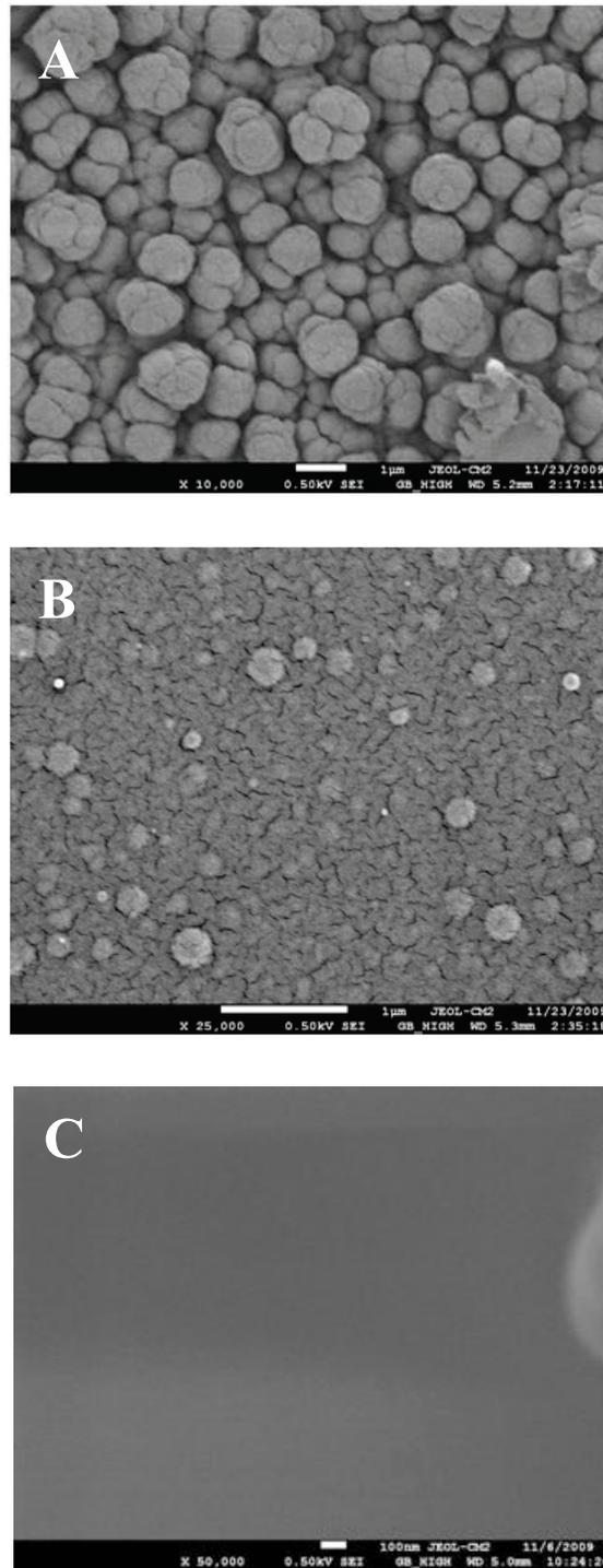
**Figure 3:** Surface morphologies of PPE:N coatings. Images of H20-PPE:N (A), H50-PPE:N (B), and L0.75-PPE:N (C) surfaces were acquired by field-emission scanning electron microscopy (FE-SEM). (After ref. [28], modified, with permission).
