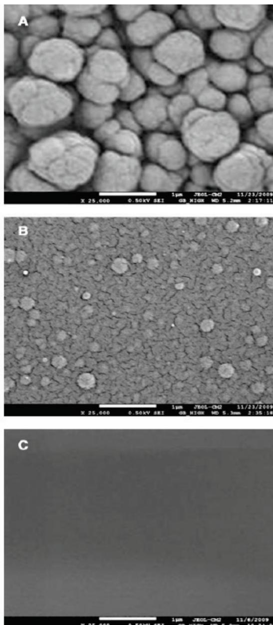
**Figure 2.** Surface morphologies of PPE:N coatings. Images of H20-PPE:N (A), H50-PPE:N (B), and L0.75-PPE:N (C) surfaces were acquired by field-emission scanning electron microscopy (FE-SEM).
