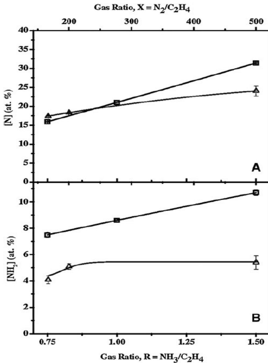
**Figure 1.** (A) Concentrations (in atomic %) of nitrogen,  $[N]$ , and (B) of primary amines,  $[NH_2]$ , in L-PPE:N (□) and H-PPE:N (Δ) deposits, as functions of the gas mixture ratios,  $R \equiv F_{NH_3}/F_{C_2H_4}$  (for L-PPE:N), or  $X \equiv F_{N_2}/F_{C_2H_4}$  (for H-PPE:N, see text).
