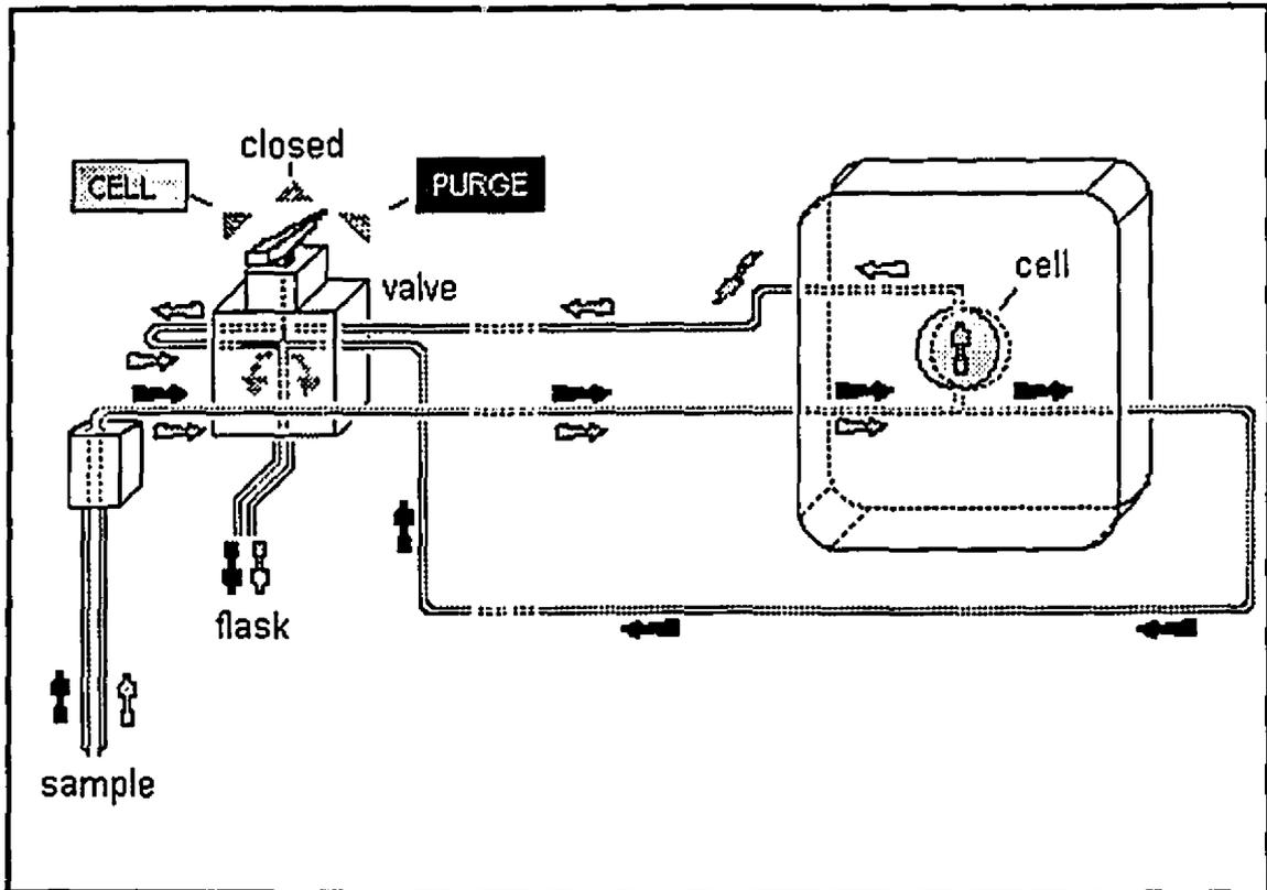
Figure 7: A Schematic Diagram of the Cell and Flow Pattern through the System.
