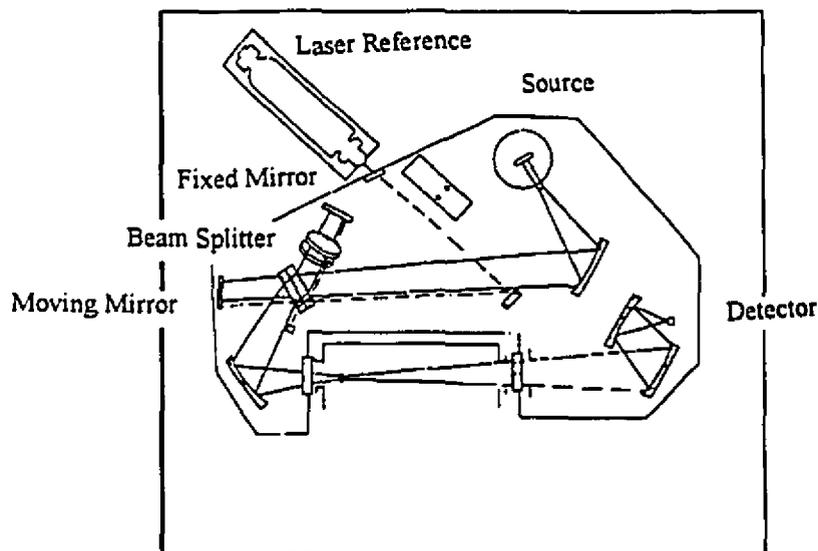
Figure 5: Single Beam FTIR Spectrometer (Source: Skoog and Leary, 1992).
