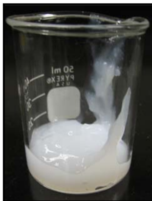
Figure 26: Typical appearance of the aluminum gel obtained by partial hydrolysis of 2M aluminum salt solutions with 5N NaOH (OH/Al 2.5).
