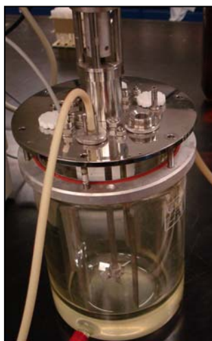
Figure 9: Applikon® reactor used for the atmospheric production of large batches of scorodite.
