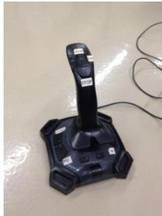
Figure 4-3: Joystick to provide desired states when HLC is not engaged.
