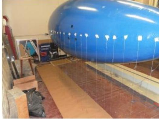
Figure 2-19: Measuring hull profile by suspending plumb-bobs
