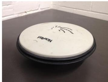
Figure 4-4: GPS base antenna
