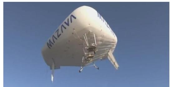
Figure 1-4: The Solar Ship [7]
