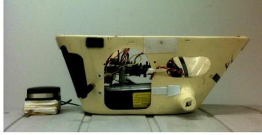
Figure 2-6: Gondola and on-board GPS antenna
