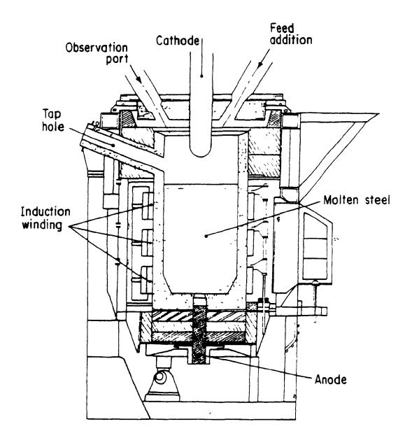
developed at the Paton Welding Institute in the U.S.S.R. (Rykalin, 1976). Rykalin (1976) also described high and low-pressure furnaces with an axial plasma torch for melting of horizontal rods as well as a furnace with radial plasma torches for the melting of bulk charges into ingots, that have been developed at the Baikov Institute of Metallurgy.
