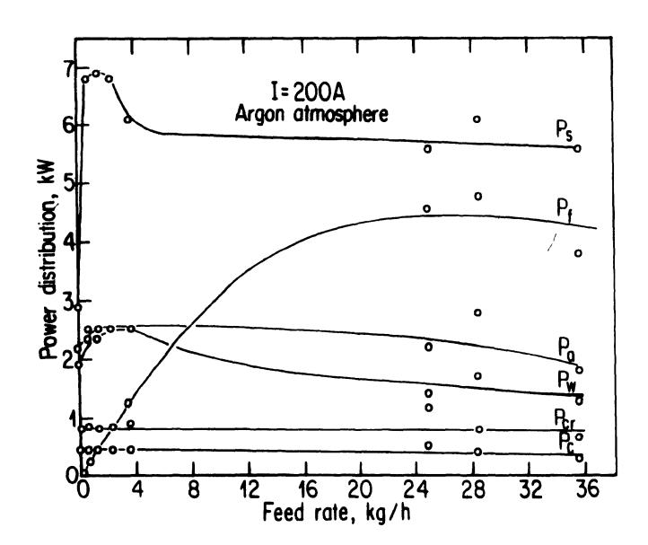
of the arc's power Therefore at higher feed rates the power transferred to the sleeve diminishes. The falling film protects and insulates the sleeve from the arc
