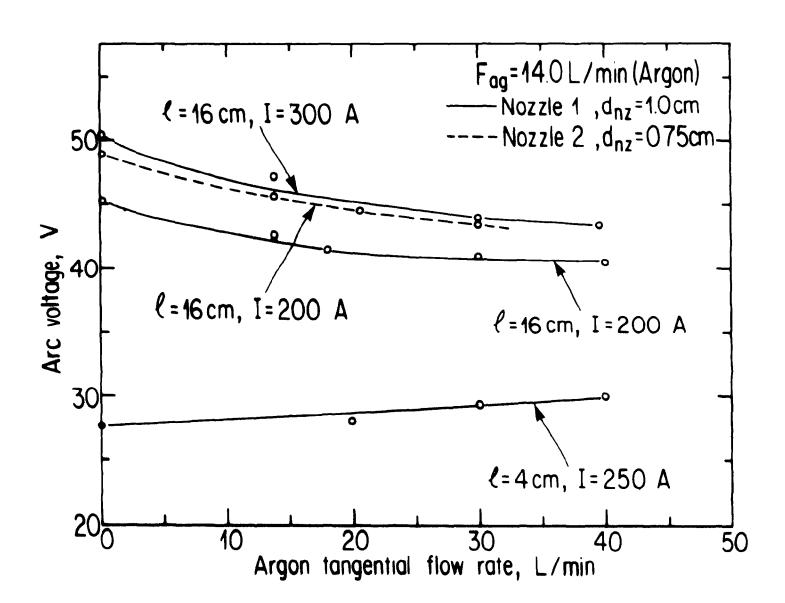
reproduce the same plots for nitrogen gas. Tsantrizos and Gauvin (1982) have shown that nitrogen is affected in the same way as argon by the above parameters except that the arc voltage is approximately double in all cases. This was confirmed in the present study. The measurements for nitrogen are tabulated in Appendix B.
