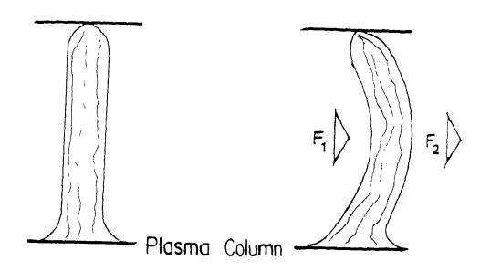
its neutral axis and the direction of the force would be such as to magnify the displacement. Thus the displacement will be emphasized and made larger until the column is extinguished.
