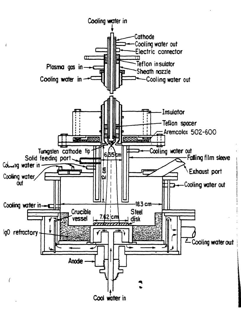
The upper opening of the sleeve was covered by a ceramic disk made of Aremcolox 502-600 machineable ceramic. An opening at the center permitted the entry of the cathode assembly. Above the ceramic, a phenolic ring insulator was used to position the cathode assembly precisely and also to electrically isolate the cathode assembly from the rest of the reactor.
