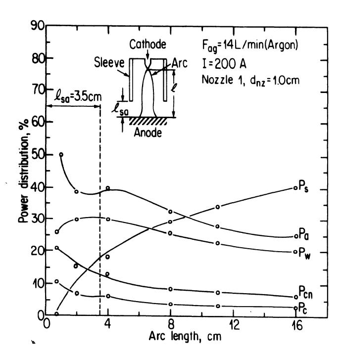
The overall trend of decreasing energy transfer to the anode with increasing arc length results from a greater portion of the arc energy being radiated by the increasingly longer arc (hence higher arc voltage) to the walls and sleeve of the reactor.
