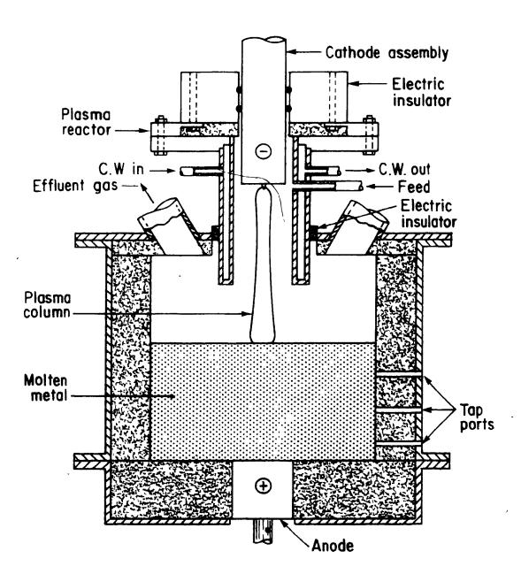
radiation from the arc. This type of reactor is very efficient as the falling film absorbs all of the radiant heat generated by the plasma arc. The other major region of heat transfer from the arc is at the anode, taking advantage of the anode fall. This serves to heat the molten pool in the bottom crucible, thus enabling it to be also used as a reaction site.
