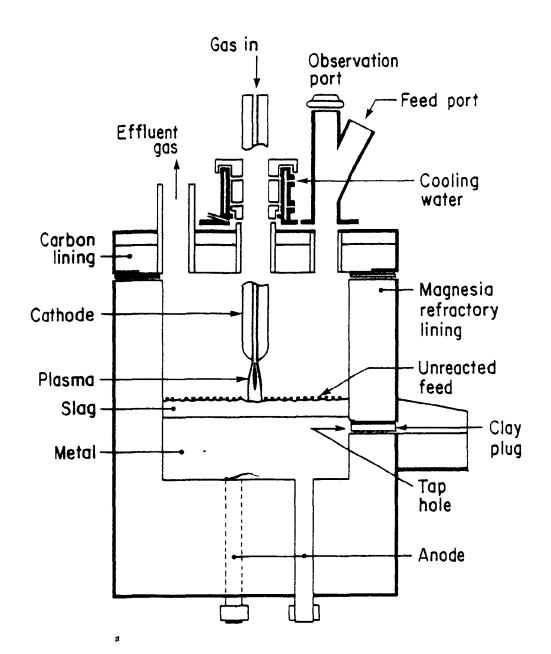
hollow graphite tathode, through which a mixture of argon and nitrogen was passed as the plasmagen gas. Based on this work. Middleburg Steel and Allovs have recently ordered a 20-MW plasma furnace from ASEA, Sweden, to be commissioned in October 1984.
