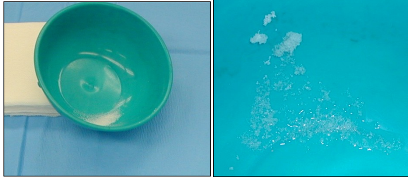
Figure- 7: White BC particles placed into a green dish (Left). A sample of BC was wet with normal saline and became ready to be packed into the chamber (right).
