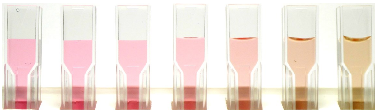
Figure 5.3 Visible change in the appearance of Compound 7 ( 10\ \mu\text{M} in \text{pH} = 7.4 buffer) on titration with dopamine ( 0 - 100\ \text{mM} ). From left to right, dopamine concentration is: 0 , 1 , 5 , 10 , 25 , 50 , and 100\ \text{mM} .
