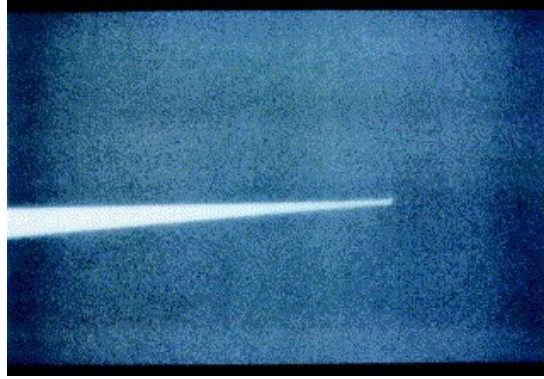
Figure 1.26 A scanning electron micrograph of a pulled fibre tip. The tip diameter is approximately 50 nm. Reproduced from Reference 223 with permission from Elsevier, copyright 2000.
