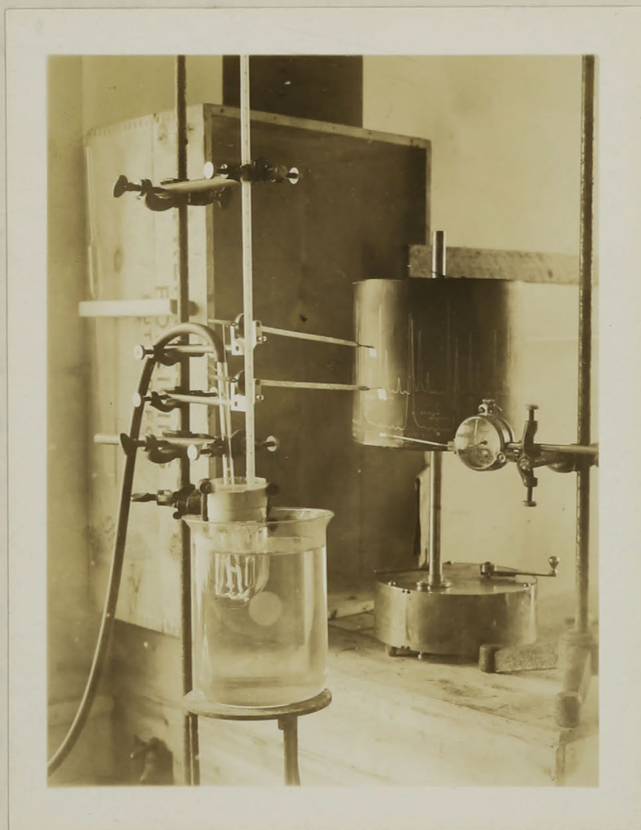
Photograph showing the general arrangement of the apparatus as used in the experiments on isolated strips taken from the gastro-intestinal tract.
