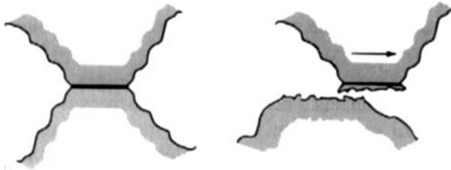
Figure 2.1 Schematic of adhesive wear [135]. Material is transferred from one surface to the other through adhesion Fatigue and delamination wear occurs through repeating loading and unloading of a surface at stress levels in the material where the load cannot be sustained for multiple loadings. Wear debris are formed when fatigue cracks cause liberation of the surface material (see Figure 2.2a). In sliding
