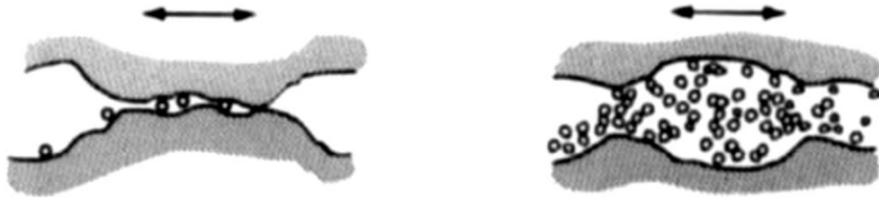
Figure 2.4 Schematic of chemical wear [135]. Oxide particles are removed from the surface. The oxide layer is then reformed and removed again.
