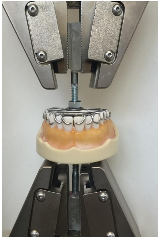
Supplemental Figure 7.2. Experimental design for measuring retention force of circumferential clasps engaging teeth.
