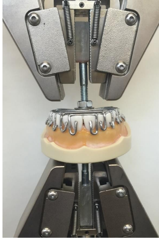
Supplemental Figure 7.3. Experimental design for measuring retention force of I-bar clasps engaging teeth.
