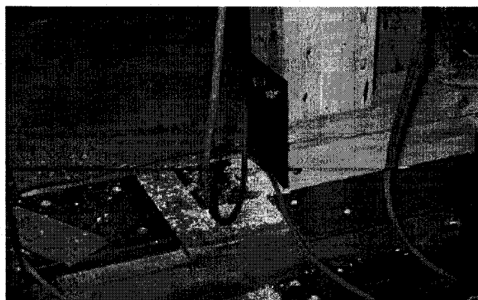
Figure 9. Additional tie-down used on Wall No. 8.
