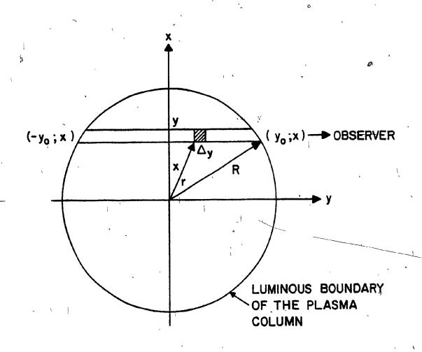
The observed specific intensity  $\underline{I}_{\lambda}(x,z)$  represents an integral of the emission through the plasma because of the gradient of  $\underline{\varepsilon}_{\lambda}$  (i.e., temperature). At constant  $\underline{x}$ :
