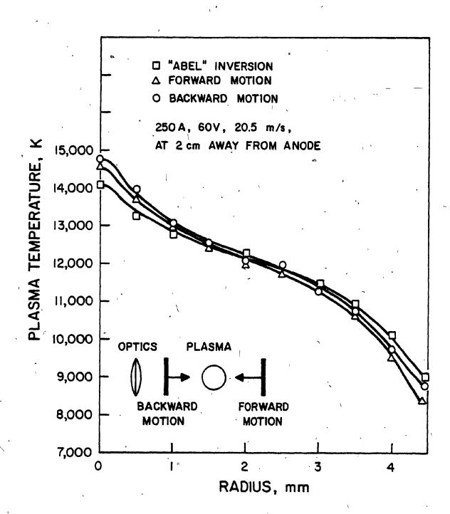
emission coefficients for 4806 Å and 6965 Å lines. The coefficients given by Barr (1962) (discussed in Appendix A) were used in the program. The temperatures obtained from the emission coefficients via Equation (1) or (2) (depending on the range) were compared with the values obtained by the "sweeping blocking element" technique.
