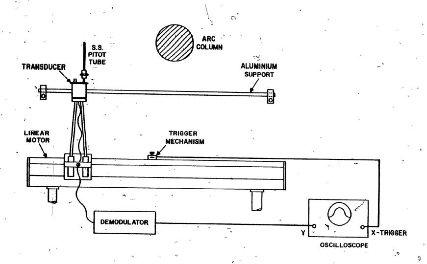
whose output was displayed on a Gould-Brush digital storage oscilloscope. The same triggering system as in the temperature diagnostic system was also employed here. The transducer and the pitot tube were calibrated against an accurate alcohol manometer.
