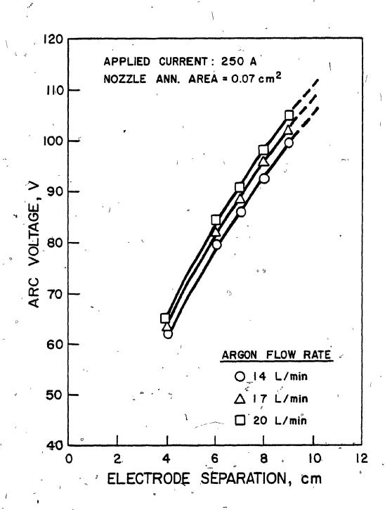
ARC VOLTAGE VARIATION WITH ELECTRODE SEPARATION
