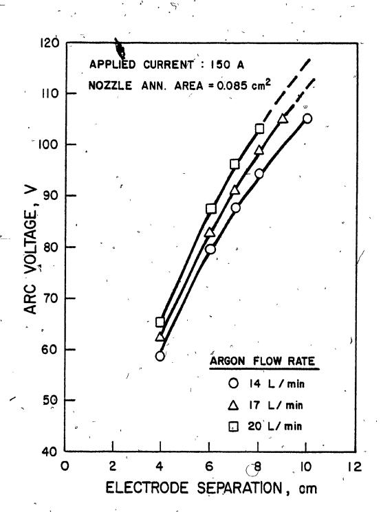
ARC VOLTAGE VARIATION WITH ELECTRODE SEPARATION
