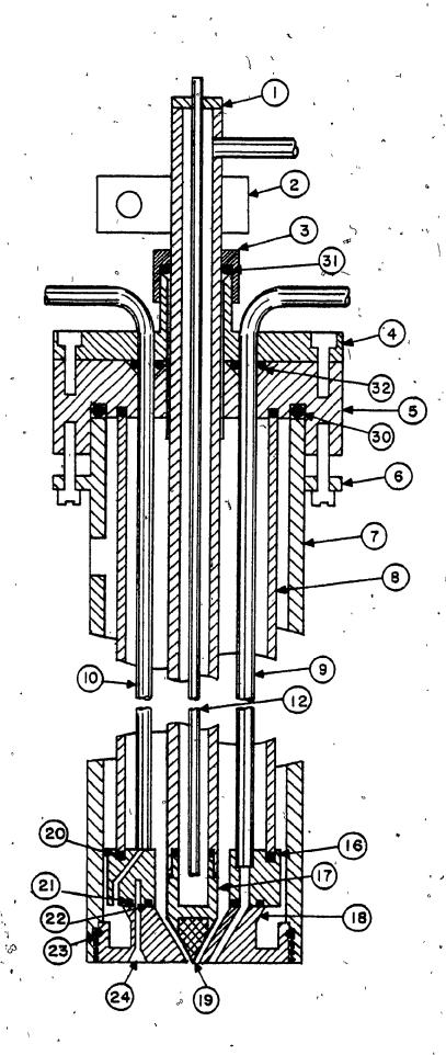
gas feeds, the end caps close the assembly at the top and help support the long feed tubes. The cathode-cooling system was designed to give maximum cooling in the form of an impinging water jet. The pressure drop calculations dictated the size of tube diameters to be used. Table B-I gives the materials of construction as well as the important dimensions of the parts of the cathode assembly shown in Figure B-1.
