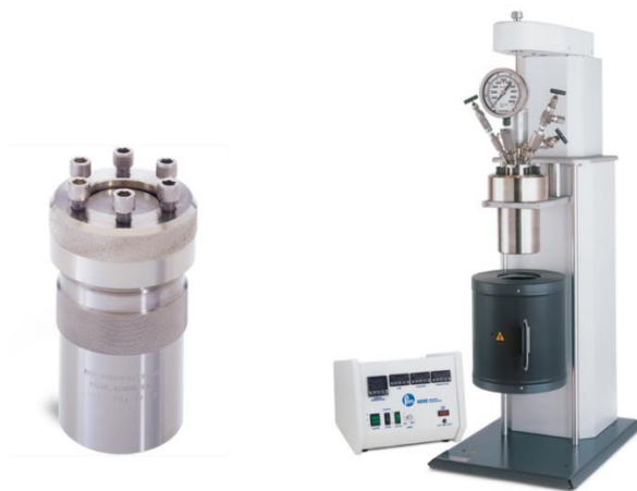
Figure 2.10. Typical reactors for hydrothermal synthesis. On the left is a simple closed-vessel that can be heated in an oven, while on the right is a more complex autoclave equipped with temperature and pressure sensors and a stirrer, which is heated by a heating mantle with temperature control. 89
