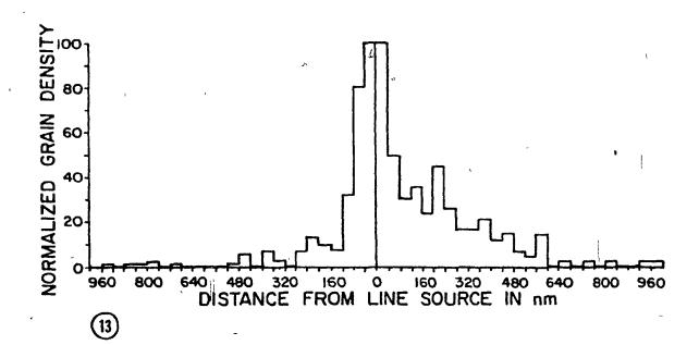
Figure I-14 A histogram of the normalized grain distribution on either side of a  $^{125}$ I line source is shown. The radioautographs were exposed after dipping in Ilford L4 emulsion and were then developed in Kodak D19b. The silver grains formed were of the filamentous type. No significant (p = 0.05) difference was found by  $\chi^2$  between normalized grain counts per unit distance from the source, over the Epon and celloidin sides of the line.
