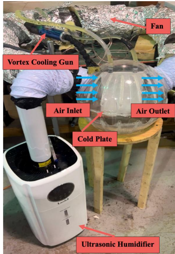
Figure 3.2. Photograph of the overall experimental setup to show instrumentation and data logging positioning. Blue arrows indicate the airflow rate.
