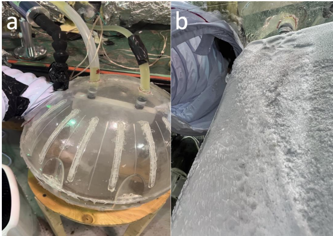
Figure 4.2. Dehumidification system overview, (a) Exterior view of the circular chamber with a cold plate installed inside, (b) Interior view showing ice crystals formed on the surface of the cold plate.
