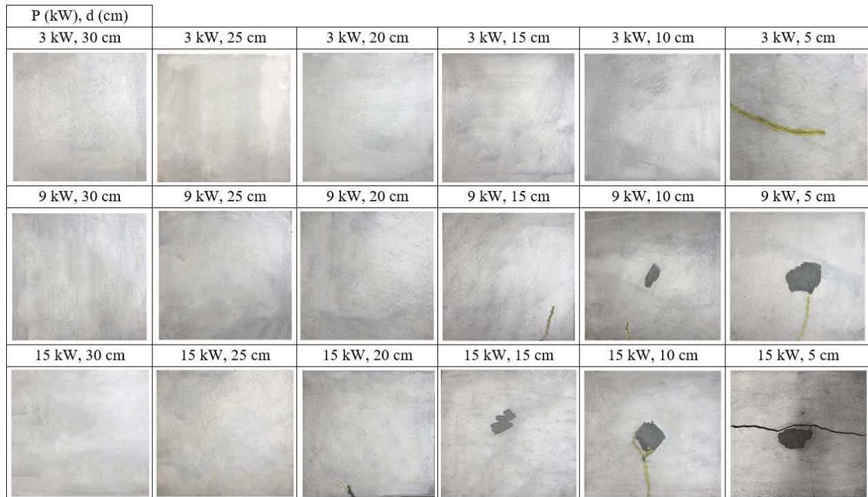
Figure 5.6: Illustration of visible crack development at the surface of the topmost basalt specimens irradiated at 60 s microwave exposure and different power levels and distances from the horn antenna
