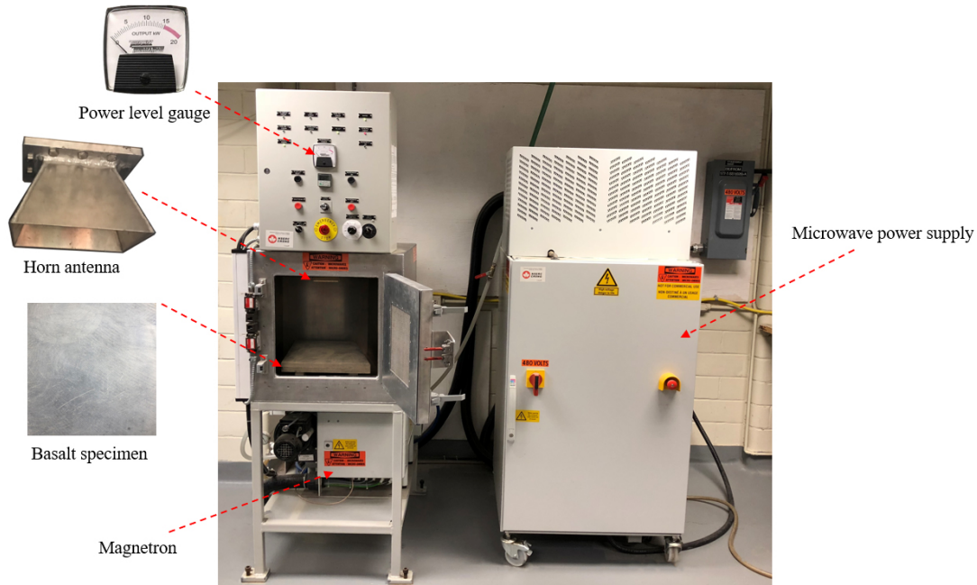
Figure 5.1: Industrial single-mode, variable high-power (up to 15 kW) microwave cavity system in the Geomechanics Laboratory at McGill University
