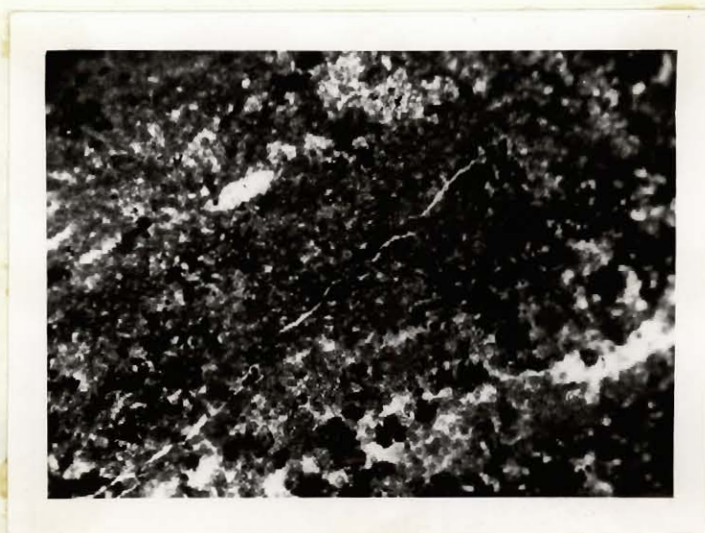
PLATE 36. Microphotograph of thin section of Iron-rich bed of Thinly-bedded Chert iron formation west of Strain Lake. x 270, ordinary light.
