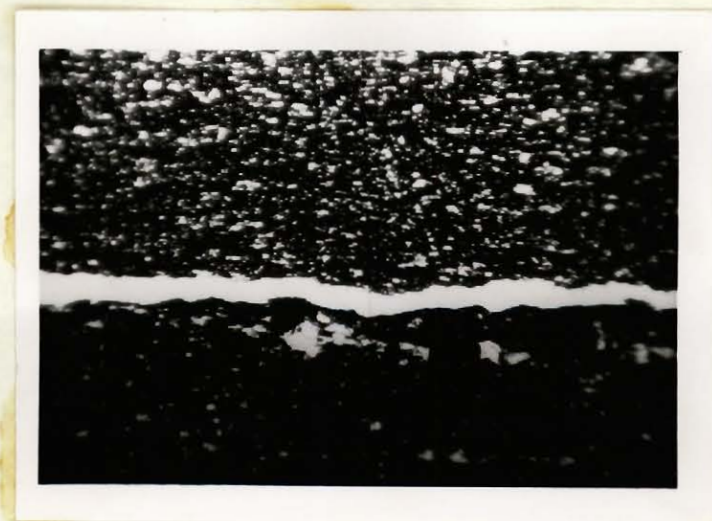
PLATE 64. Microphotograph of thin section of graphite shale east of Teeter Lake. x 18, ordinary light.
