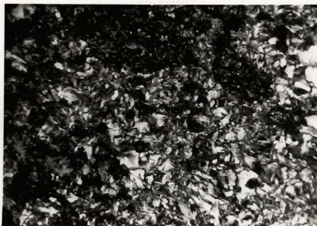
PLATE 50. Microphotograph of thin section of Carbonate iron formation east of Irony Lake, showing fibrous minnesotaite in chert groundmass. x 60, polarized light.
