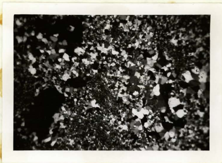
PLATE 51. Microphotograph of thin section of Spotted Silicate iron formation east of Irony Lake. x 60, polarized light.
