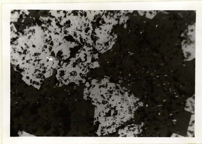
PLATE 41. Microphotograph of polished section of Magnetite iron formation east of Irony Lake. x 60, Magnetite - grey Hematite - light grey
