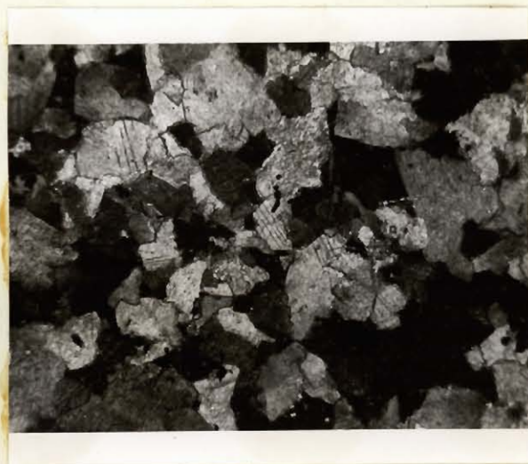
PLATE 45. Microphotograph of thin section of massive iron carbonate material of Carbonate iron formation east of Irony Lake. x 60, polarized light.
