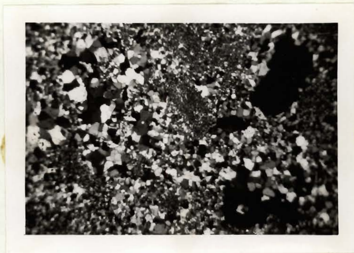
PLATE 38. Microphotograph of thin section of fine-grained chert layer typical of those rocks found west of Strain Lake. x 60, polarized light.
