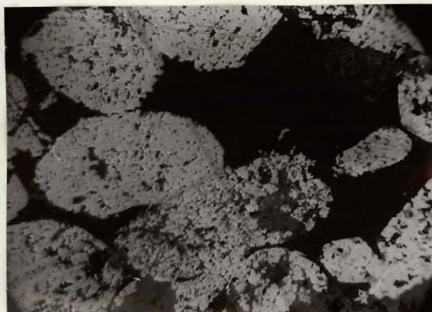
PLATE 25. Microphotograph of polished section of Cherty Metallic iron formation west of Strain Lake. x 60, grains of magnetite.
