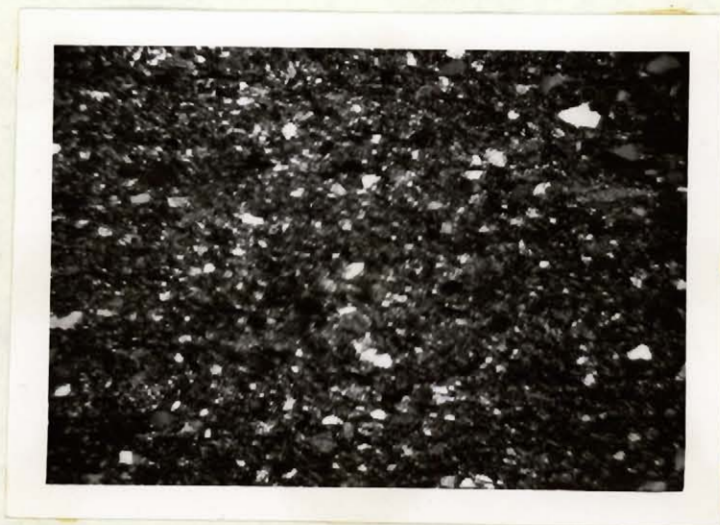
PLATE 55. Microphotograph of thin section of Chioack greywacke south of Finger Lake. x 18, polarized light.
