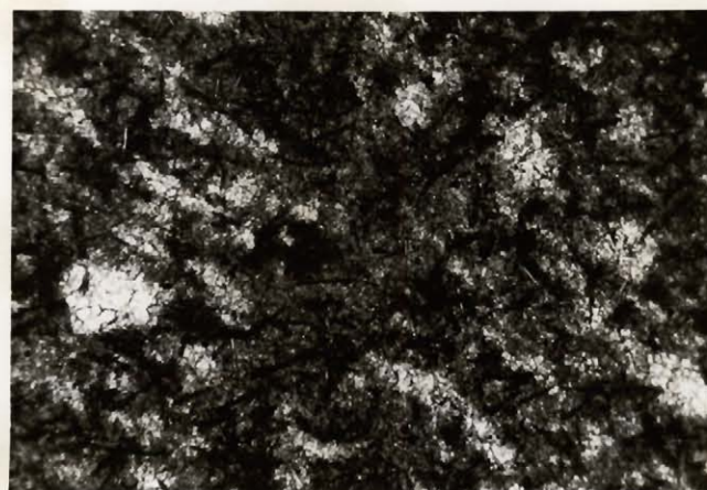
PLATE 43. Microphotograph of thin section of Blue Weathering Carbonate iron formation east of Irony Lake. x 60, polarized light. Groundmass of iron carbonate with black prismatic veins of stilpnomelane.
