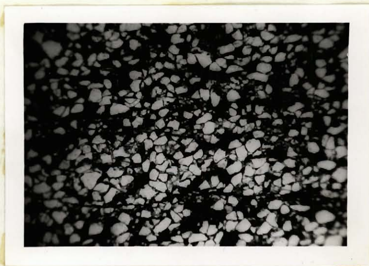
PLATE 56. Microphotograph of thin section of Chioack red sandstone west of Strain Lake. x 18, ordinary light. Note: Dark matrix which gives red colour to the rock.
