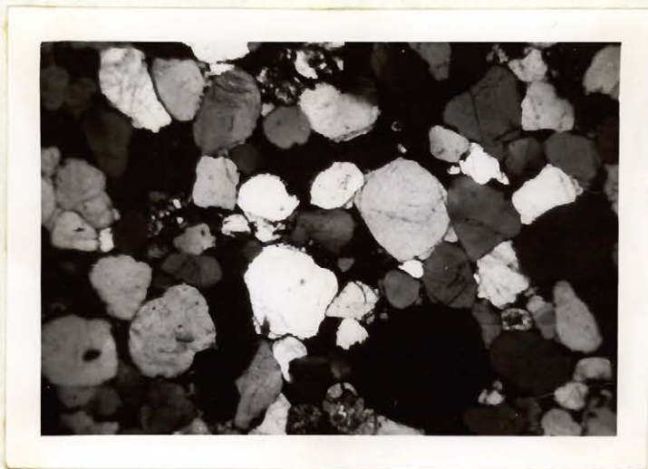
PLATE 18. Microphotograph of thin section of Alison quartzite, x 18, polarized light.
