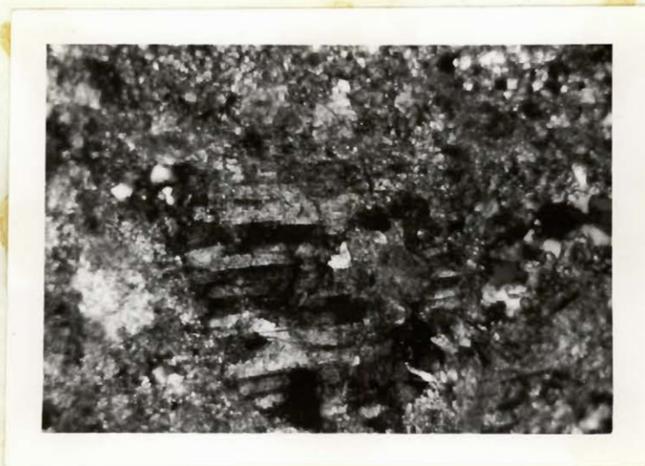
PLATE 52. Microphotograph of thin section of Carbonate spot in Spotted Silicate iron formation east of Irony Lake. x60, ordinary light.
