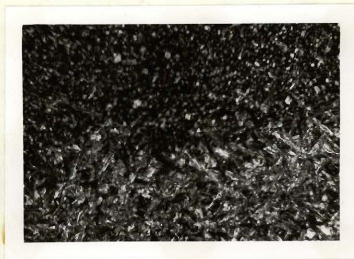
PLATE 42. Microphotograph of thin section of Carbonate iron formation, east of Irony Lake showing chert layer iron silicate layer boundary. x 60, polarized light.
