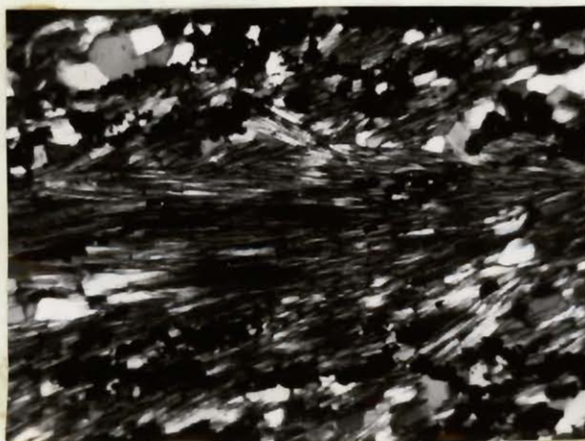
PLATE 34. Microphotograph of thin section of Cherty Metallic iron formation north of Finger Lake. x 60, polarized light. Note fibrous cummingtonite in chert groundmass.
