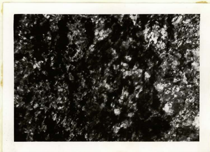
PLATE 40. Microphotograph of thin section of Thin-bedded Carbonate iron formation west of the West Arm of Finger Lake. x 60, polarized light.
