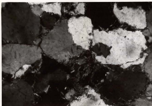
PLATE 20. Microphotograph of thin section of Alison quartzite west of the North Arm of Finger Lake. x 60, polarized light. Note needles of stilpnomelane cutting the edges of the quartz grains.
