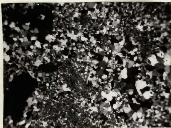
PLATE 32. Microphotograph of thin section of chert layer of Cherty Metallic iron formation west of Strain Lake. x 60, polarized light.
