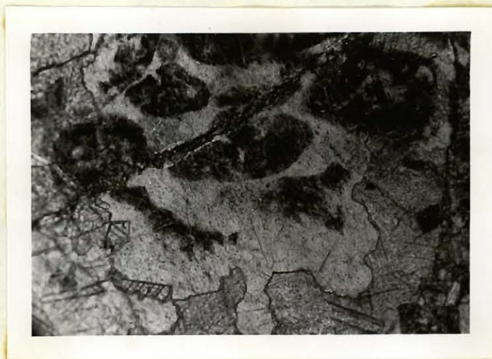
PLATE 47. Microphotograph of thin section of Carbonate iron formation east of Irony Lake. x 60, ordinary light. Note: Granule structure indicated by "dust-like impurities".
