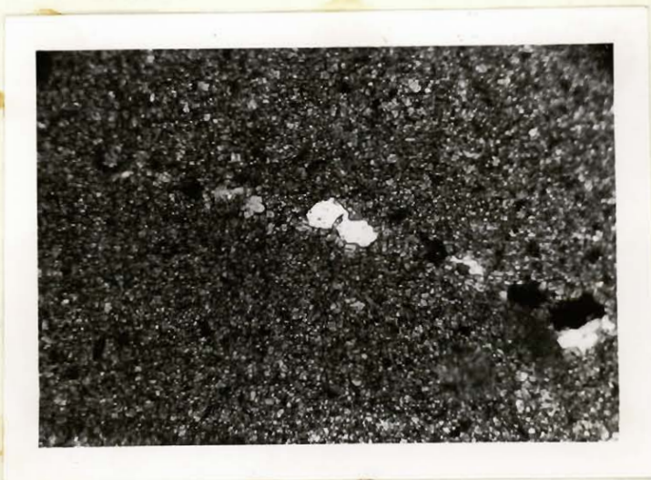
PLATE 63. Microphotograph of thin section of Abner dolomite east of Teeter lake. x 18, polarized light. Note: Quartz stringer.
