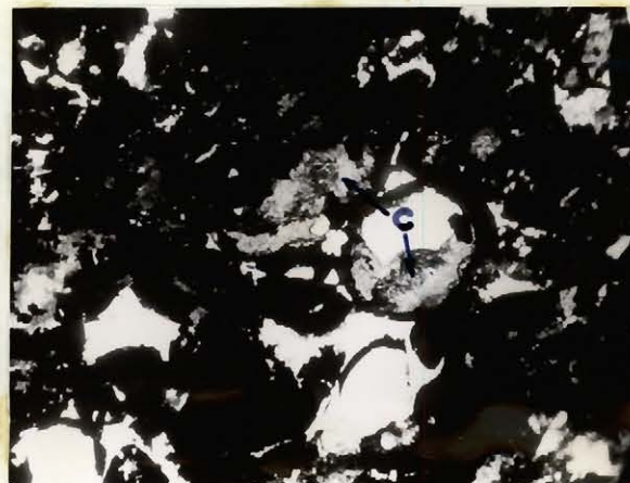
PLATE 31. Microphotograph of thin section of iron chlorite (c) filling granule of magnetite, from Cherty Metallic iron formation west of Strain Lake. x 60, ordinary light.
