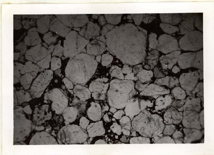
PLATE 17. Microphotograph of thin section of Alison quartzite, x 18, ordinary light.
