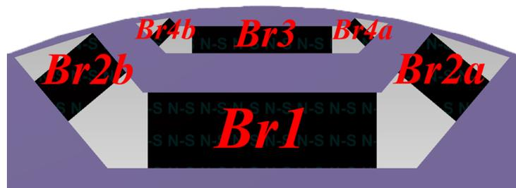
**Figure 55. Remanent Flux Density Parameters of 6 PMs across 1 Rotor Pole**
