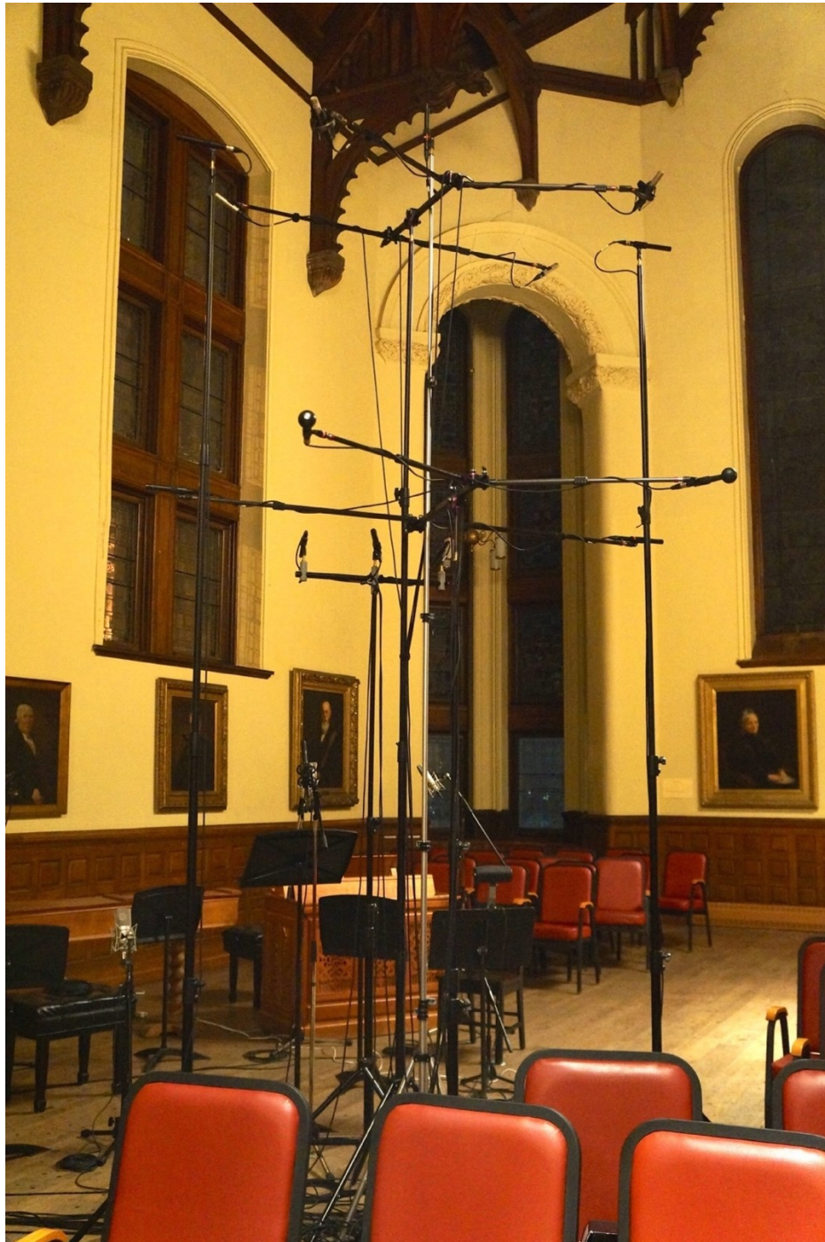
Figure 19: Microphone arrays setup for recording
