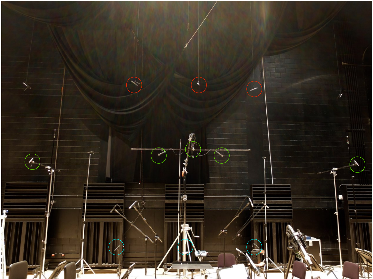
Figure 39: Frontal sound capture microphones, as seen from viola section. Red = height layer, green = main layer, blue = bottom layer.
