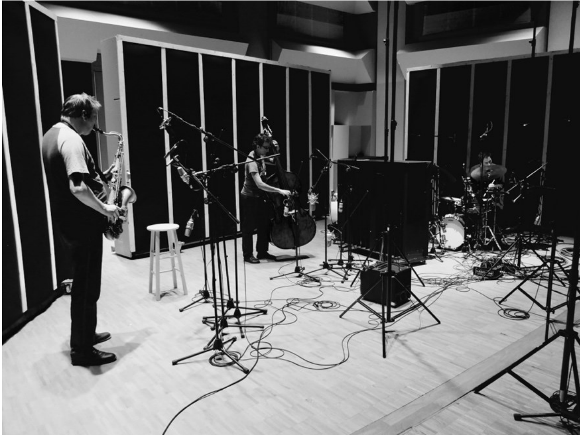
Figure 50: Jazz trio in concert hall with direct sound microphone arrays
