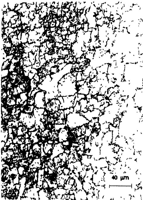
Figure 4.1 Austenite microstructure after reheating at 850°C for 10 minutes followed by a deformation of 20%
