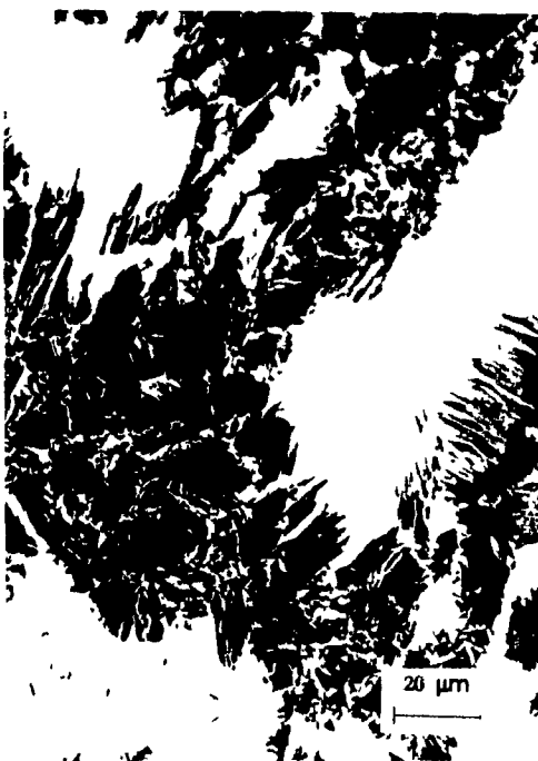
Figure 4 18 Microstructure of a specimen reheated at 800°C (in the intercritical range), deformed 20% and cooled at 90°C/s to 400°C
