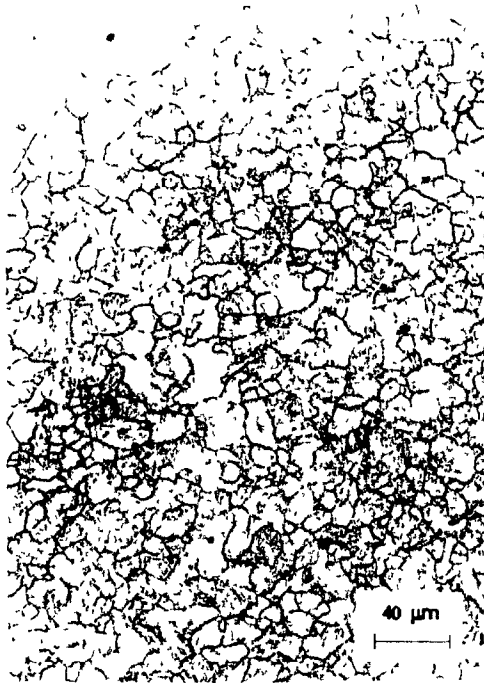
Figure 4.3. Austenite microstructure after reheating at 850°C for 10 minutes followed by a deformation of 80%
