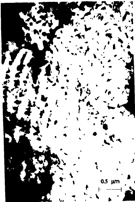
Figure 4.22 Carbides in ferrite in a specimen reheated at 1050°C and cooled at 55°C/s to 500°C
