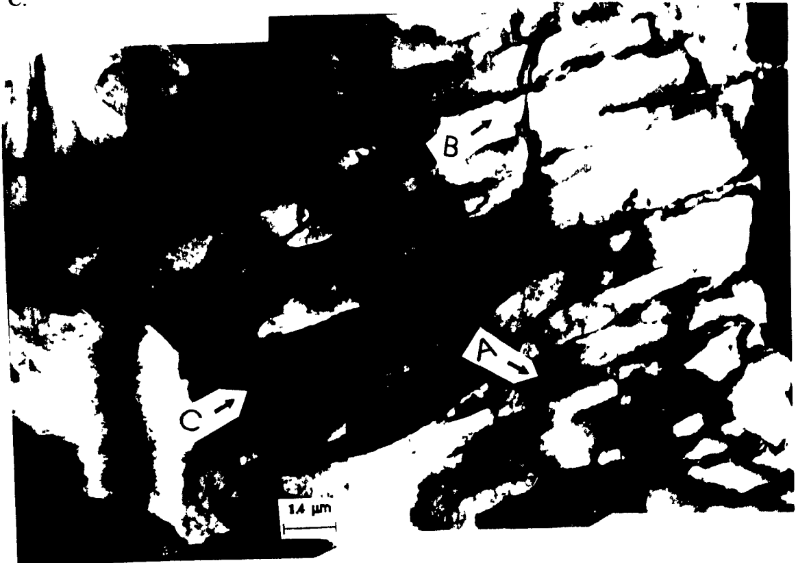
Figure 4 16 Bainites in a specimen reheated at 900°C and cooled at 90°C/s to 300°C
