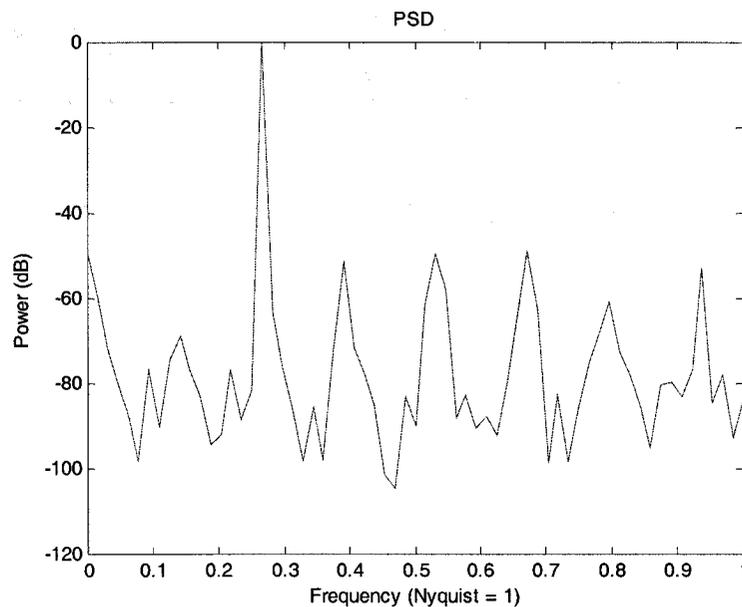
Figure 5.7: Power spectral density plot of the digitized signal using probabilistic digitization process without “zooming”.
