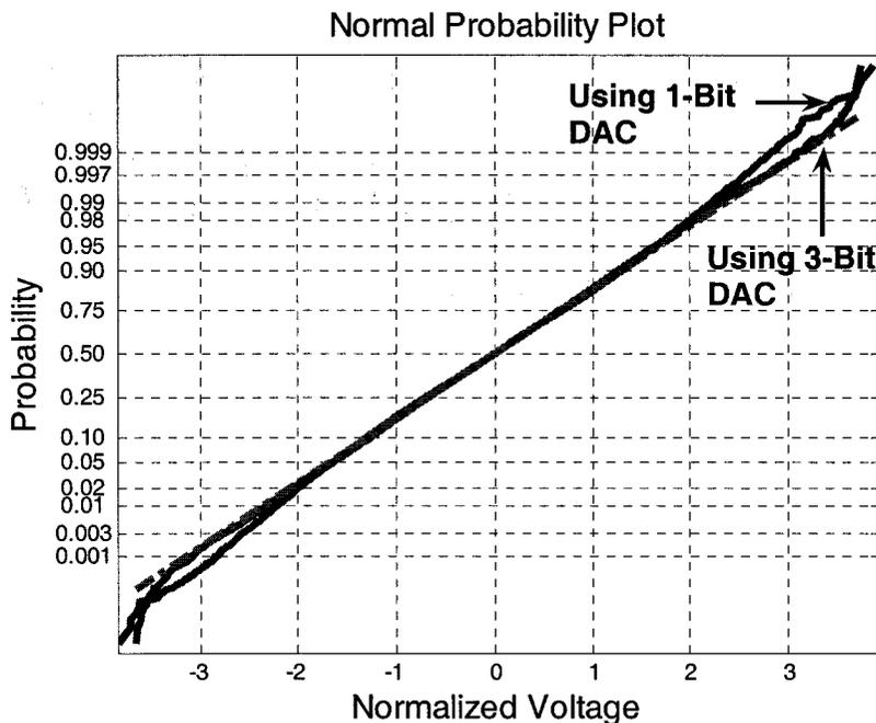
Figure 4.6: Normalized normal probability plot for a  $\sigma$  of 0.15 V, an OSR of 32 and 100 000 collected points. Two cases are shown: 1-bit and 3-bit DAC implementations.
