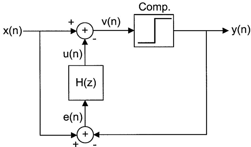
Figure 2.4: General delta-sigma modulator structure with unity signal transfer function.
