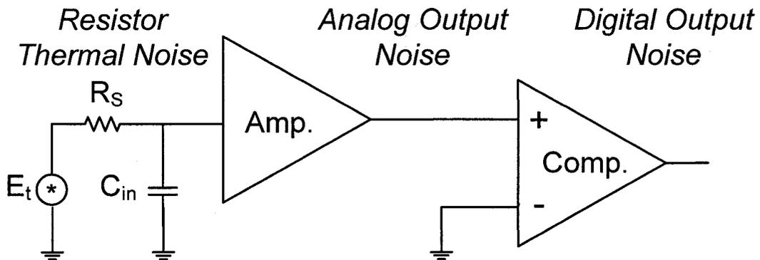
Figure 3.3: Topology of resistor thermal noise amplification method.
