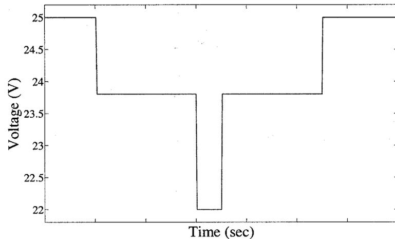
Figure 6.2: Voltage dip test signal for a 25 V load.
