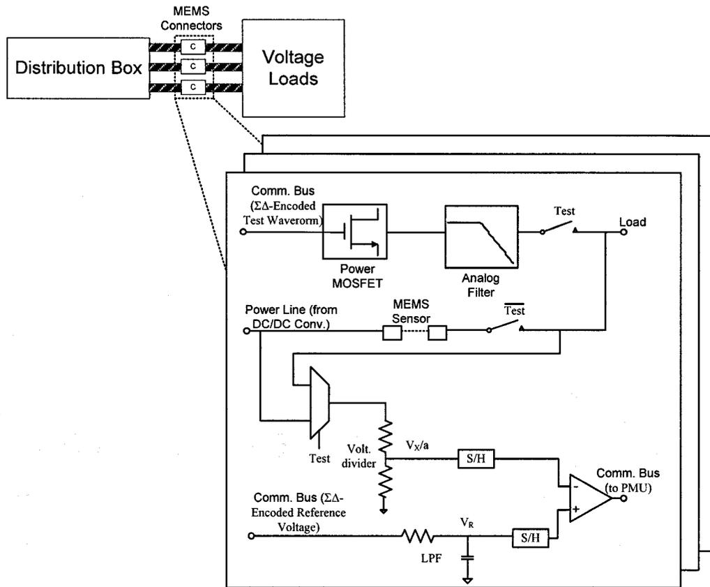
Figure 6.7: Test instrument inside MEMS connectors
