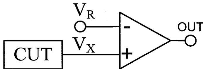
Figure 5.4: Comparator connections for probabilistic digitizer.
