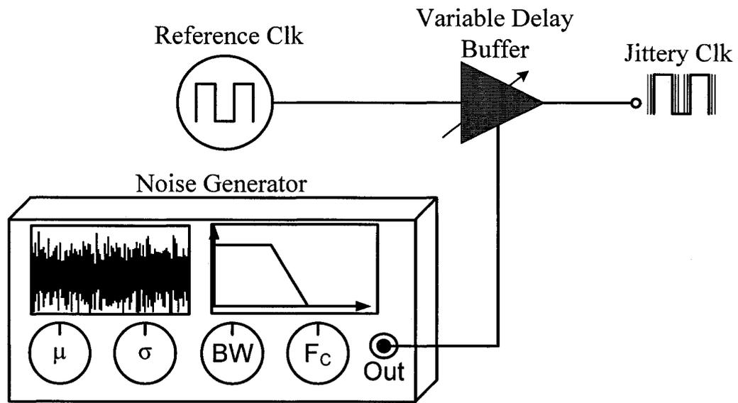
Figure 7.2: Proposed jittery clock source implementation.
