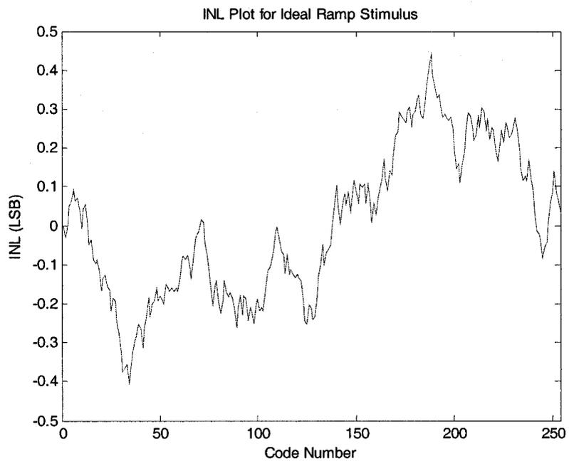
Figure 5.3: Top plot shows the INL results for a Gaussian input when 4M points are used. Bottom plot shows the real INL results for an ideal ramp.
