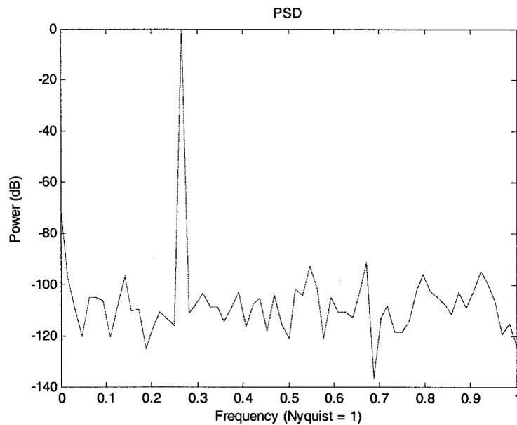
Figure 5.8: Power spectral density of the digitized signal when “zooming” technique is used to enhance the resolution.
