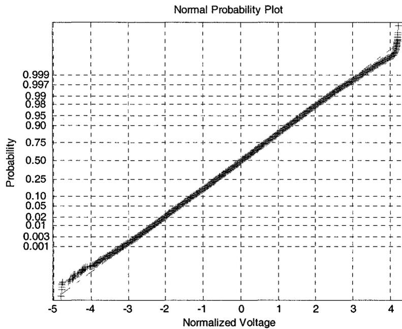
Figure 4.9: Experimental normalized normal probability plot of captured signal when filter has a bandwidth 10 times the nominal (19.5 kHz).
