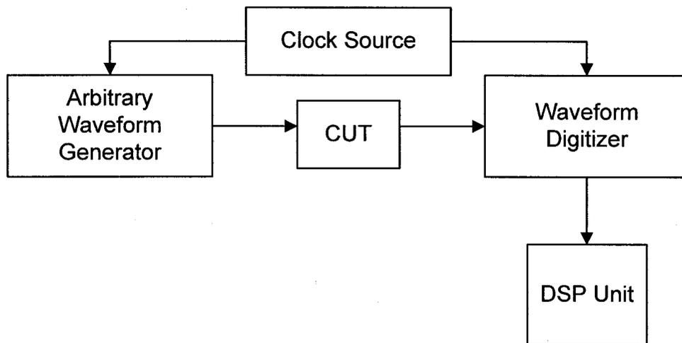
Figure 1.2: Block diagram of mixed-signal on-chip test system.
