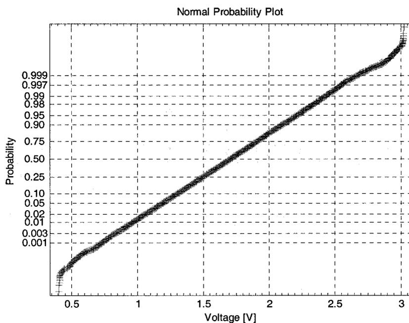
Figure 4.8: Experimental normal probability plot of captured signal when filter has a 1.95 kHz bandwidth.
