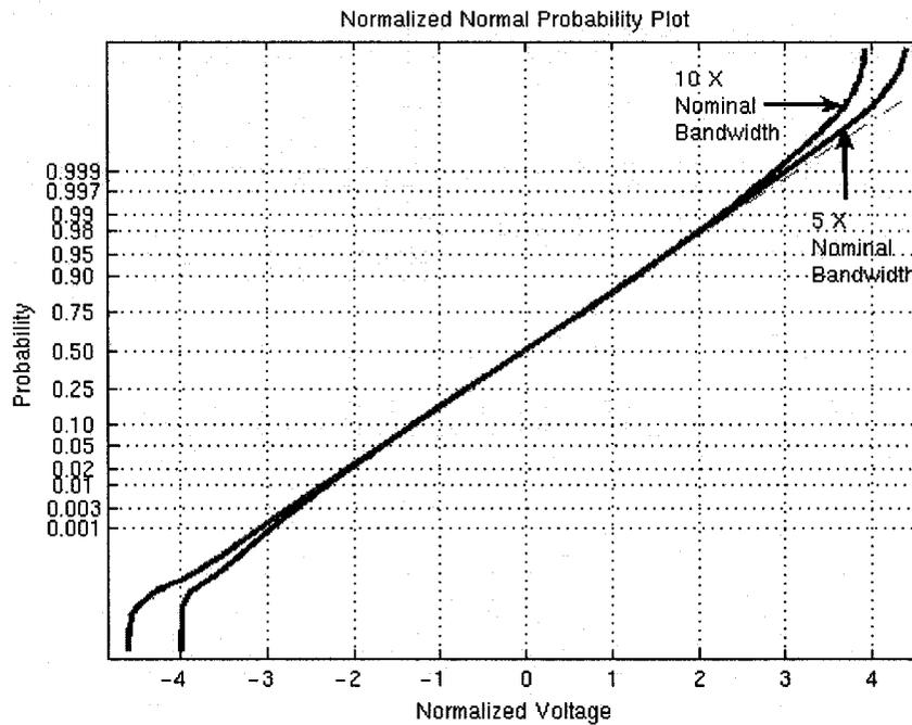
Figure 4.5: Normalized normal probability plot for an analog filter having 5 and 10 times the nominal bandwidth.
