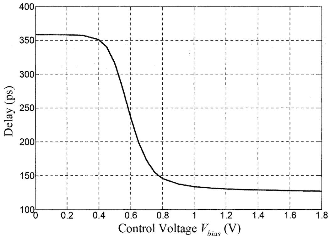
Figure 7.4: Simulated delay versus control voltage of voltage-controlled delay buffer [32].
