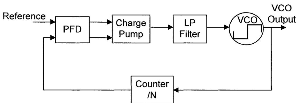
Figure 7.1: Digital phase locked loop functional block diagram.
