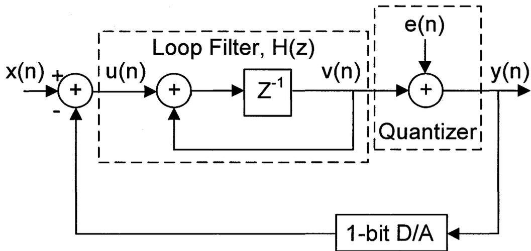
Figure 2.2: First order  $\Sigma\Delta$  modulator architecture.
