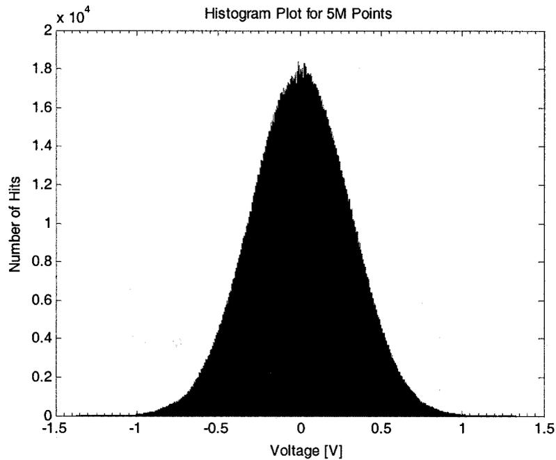
Figure 4.3: Histogram plot for 5M points and 1.95 kHz filter bandwidth.
