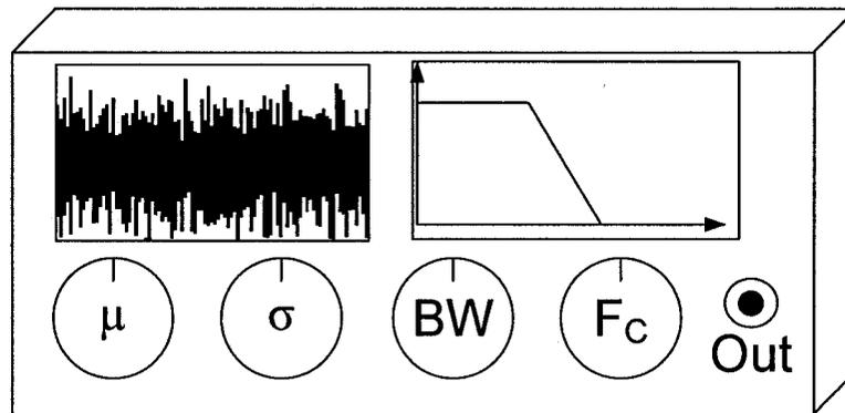
Figure 4.1: Gaussian noise source and its various knobs.
