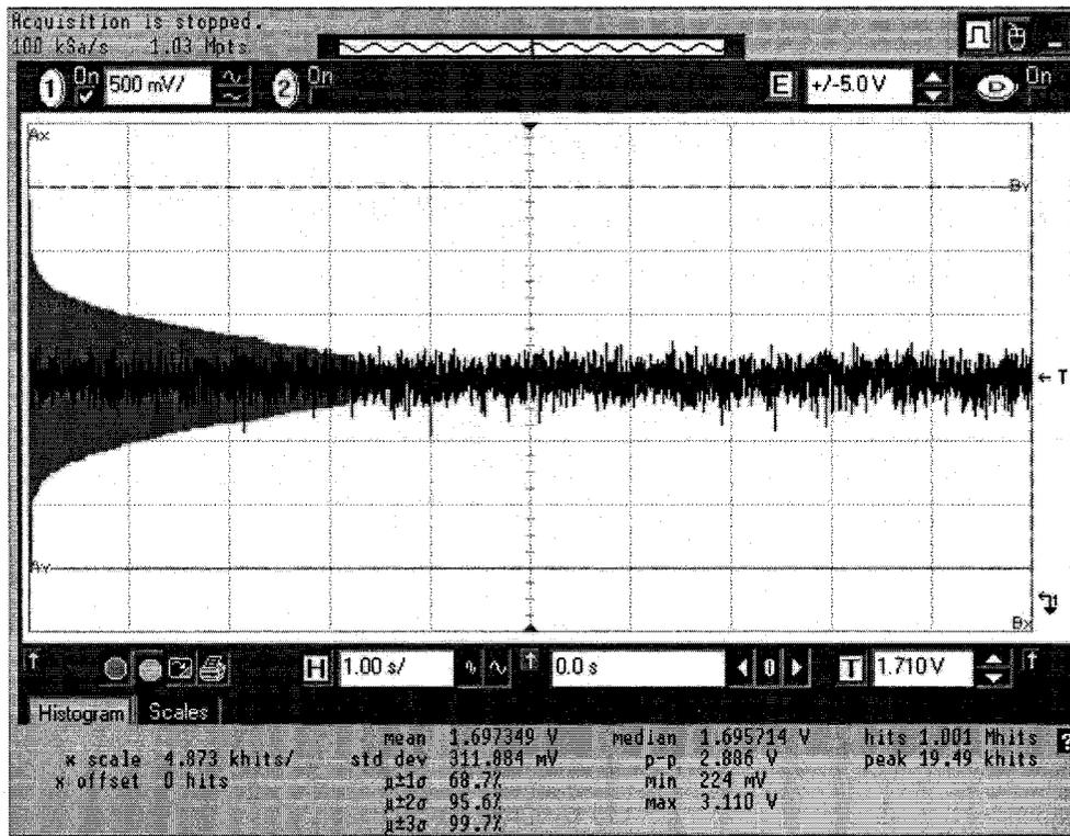
Figure 4.7: Captured generated Gaussian signal using Agilent Infiniium scope. Note that the vertically plotted histogram distribution is superimposed on the horizontally plotted time signal.
