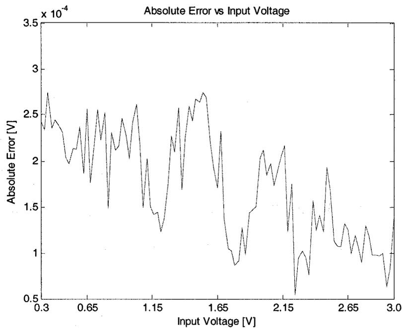
Figure 6.8: Absolute error vs input voltage level when “zooming” technique is used.
