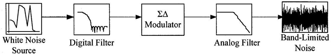
Figure 4.2: Band-limited Gaussian noise generator diagram.
