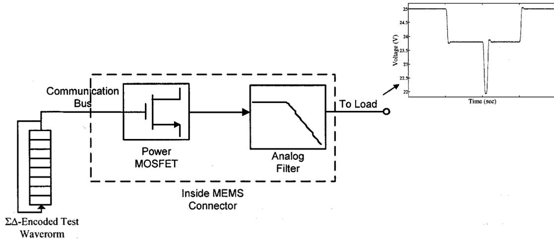
Figure 6.3: Proposed test waveform generator
