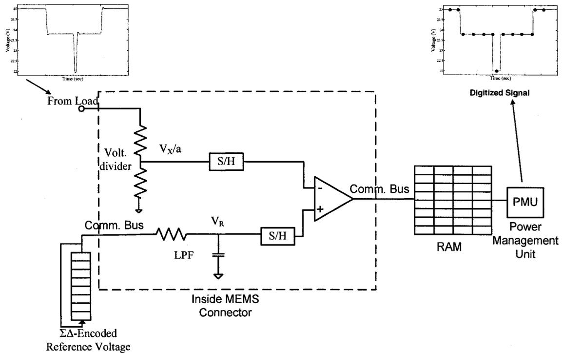
Figure 6.6: Digitizer/peak detector circuit
