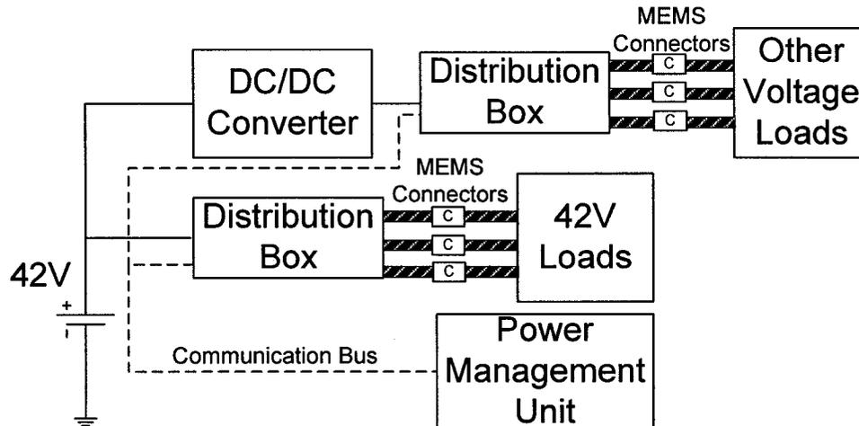
Figure 6.1: 42 V power distribution network
