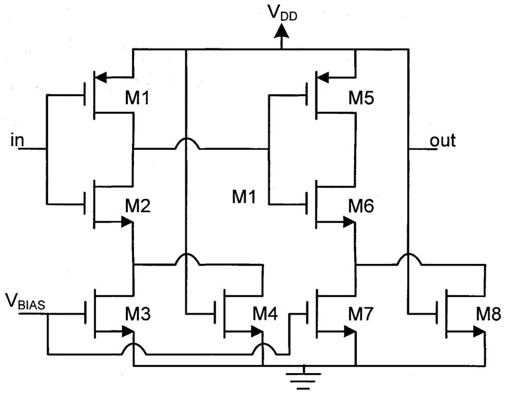
Figure 7.3: Circuit schematic for voltage-controlled delay buffer.
