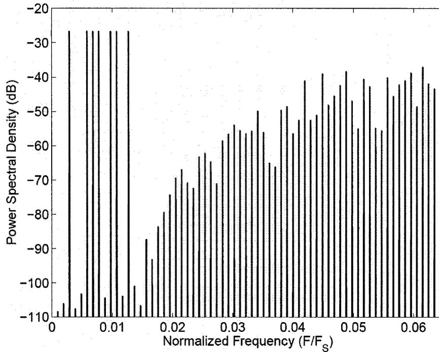
Figure 2.6: Typical spectrum of a periodically repeated finite-duration  $\Sigma\Delta$  modulated bit stream encoding a multi-tone signal [16].
