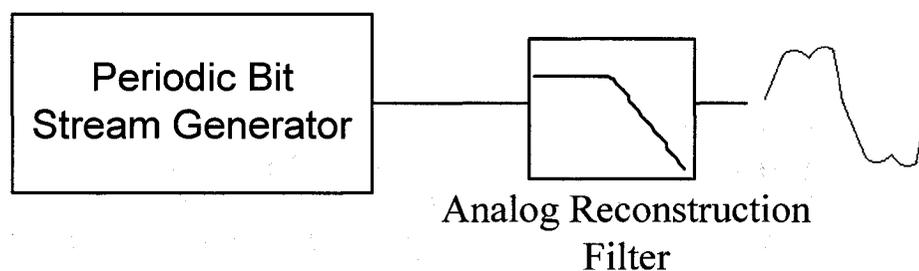
Figure 2.5: On-chip arbitrary waveform generator.
