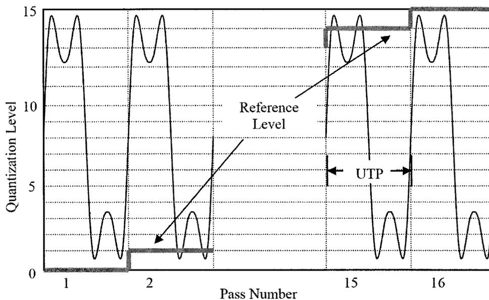
Figure 6.5: Digitization of periodic waveform [16].
