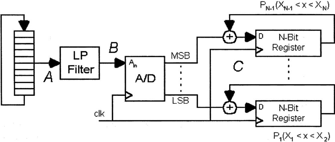
Figure 5.2: Histogram test set-up.
