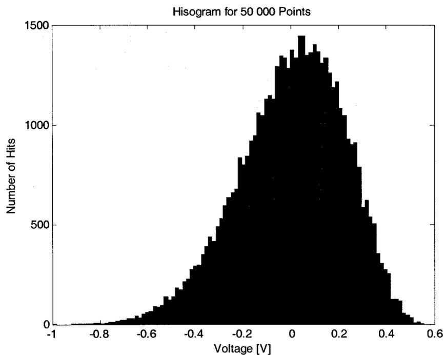
Figure 3.2: Histogram of noise signal for a 15-bit LFSR where  $V_{DD} = 1$  V and  $f_{3dB}/f_{clk} = 1/64$ .
