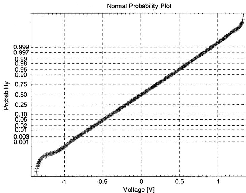
Figure 4.4: Normal probability plot for 5M points and 1.95 kHz filter bandwidth.
