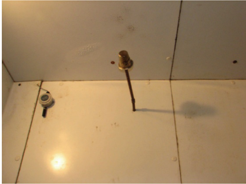
Figure 4. 34: The steam injector in the experimental cold room was located next to the temperature and humidity sensors.
