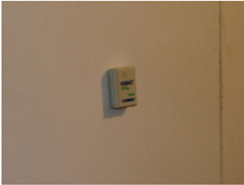
Figure 3. 21: Wall-mounted data logger recording ambient conditions in the experimental cold store.
