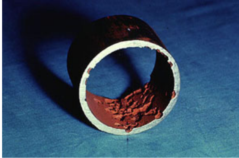
Figure 16. Tube severely damaged by oxygen [33].
