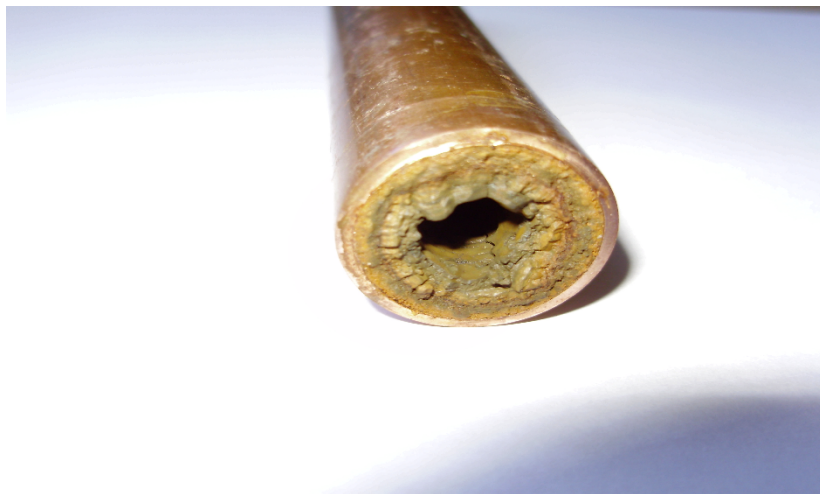
Figure 18. Boiler sludge onto the hot tube surfaces [89].
