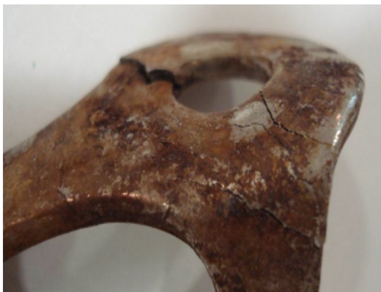
Figure 7. Stress corrosion cracking [38].
