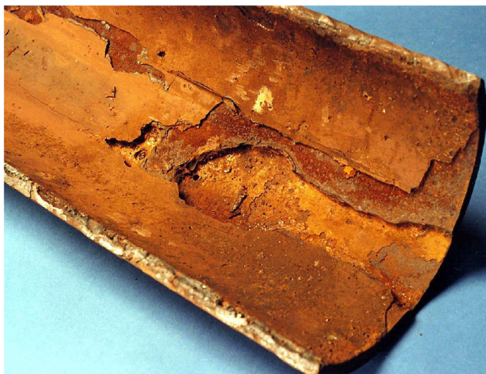
Figure 2. Pitting corrosion inside a crude oil pipeline in saltwater and carbon dioxide environment [32].
