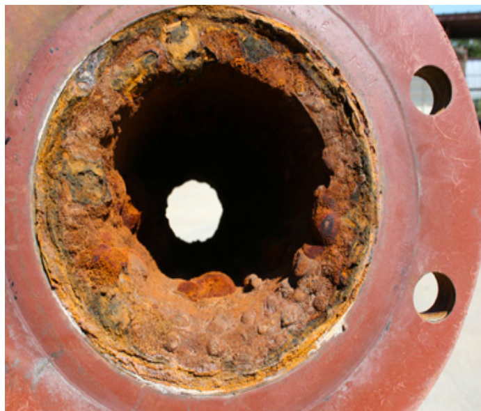
Figure 8. Microbiologically Influenced Corrosion inside the walls of a pipeline [39].
