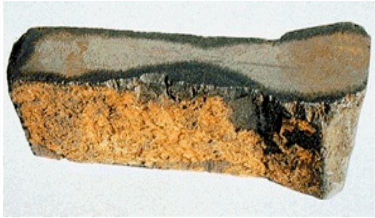
Figure 3. Dezincification of Admiralty brass [34].
