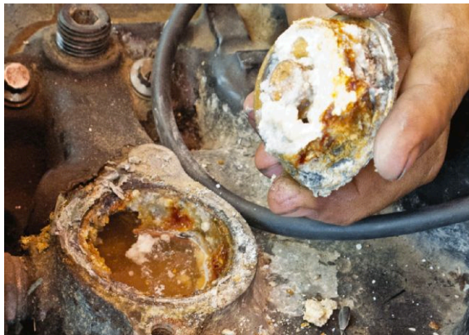
Figure 19. Corrosion in cooling system [90].
