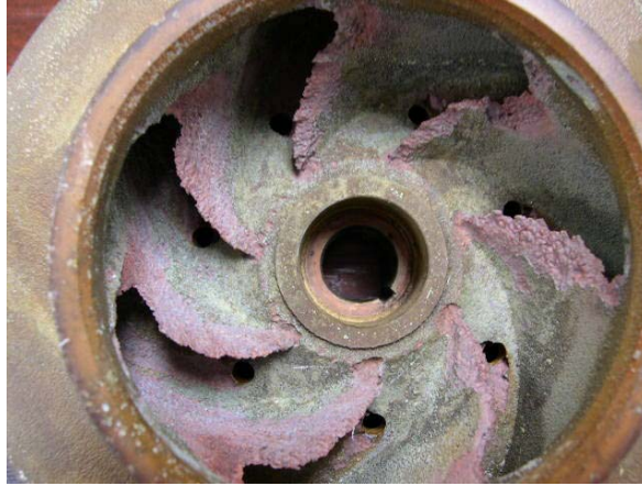
Figure 6. Corroded metal by erosion corrosion [36].
