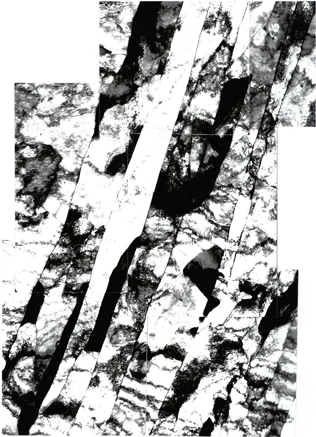
Fig. 6.32 TEM micrograph of the specimen cooled at 3.5 °C/s and shown in Fig. 6.30 (a).
