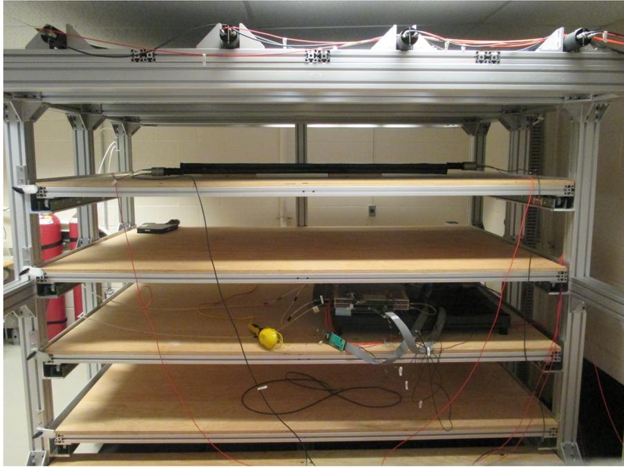
Figure 3.6: The four layers structure picture of the hodoscope.
