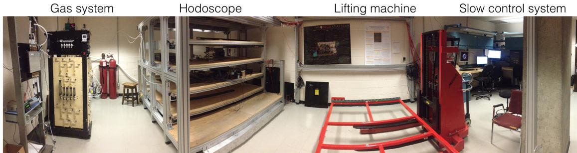
Figure 3.2: The TGC Lab in McGill. From right to left: gas system, construction where triggering system and sTGC detectors are placed, lifting jack, slow control system– work space with computers and accessories.
