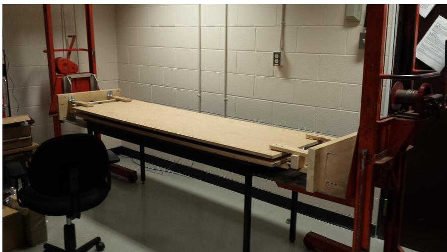
Figure 3.4: The gluing structure of scintillator and PMT.
