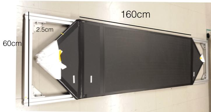
Figure 3.5: The structure of the scintillator and lightguide after wrapped in black vinyl. The size of the scintillator is  $160\text{cm} \times 60\text{cm} \times 2.5\text{cm}$
