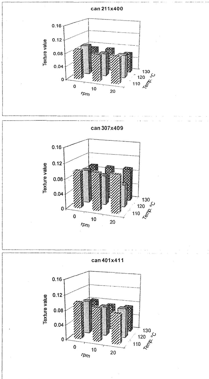
**Figure 5.7: Effects of temperature and rotational speed on texture value of canned potatoes in water**
