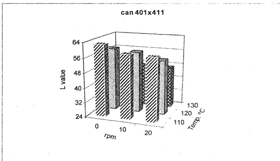
**Figure 5.2: Effects of temperature and rotational speed on L values of canned potatoes in CMC**
