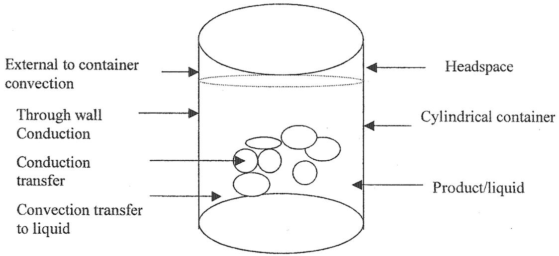
**Figure 2.2 : Heat transfer to food product in a cylindrical container (Adopted from Holdsworth, 1997)**
