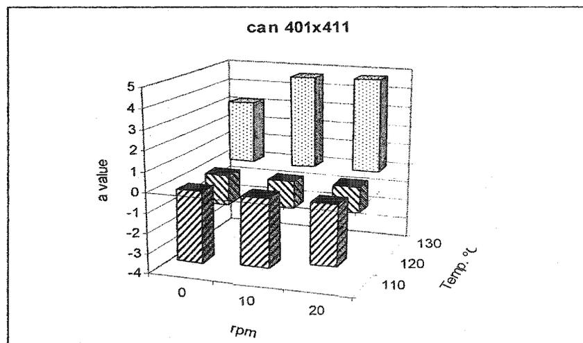
**Figure 5.3: Effects of temperature and rotational speed on 'a' values of canned potatoes in water**
