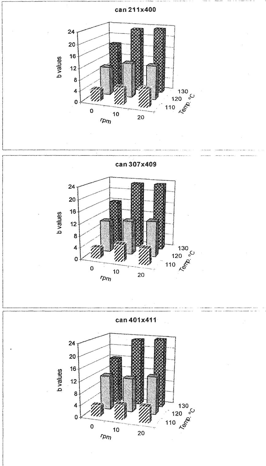
Figure 5.5: Effects of temperature and rotational speed on b values of canned potatoes in water
