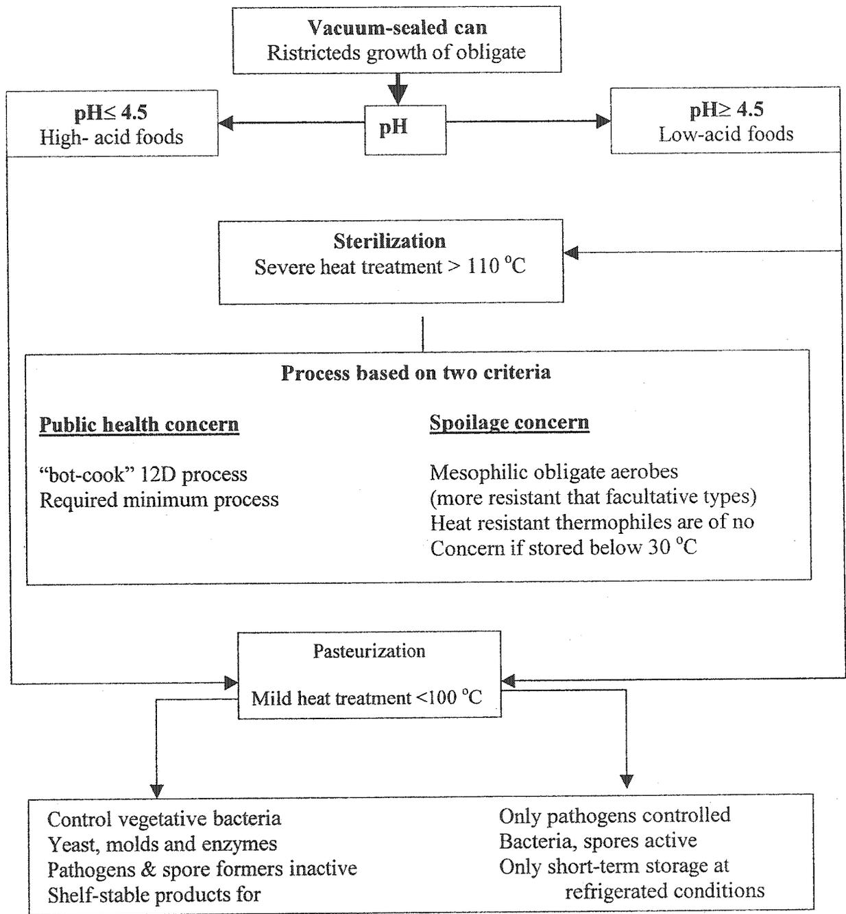
**Figure 2.1** A schematic illustrating the principles involved in thermal process applications (Source: Ramaswamy and Abbatemarco, 1996)
