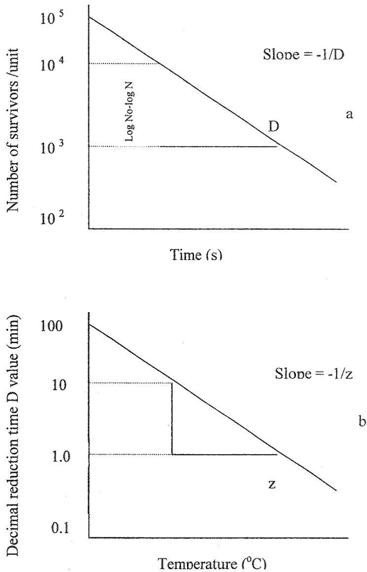
**Figure 2.4: Typical D and z value curves**
