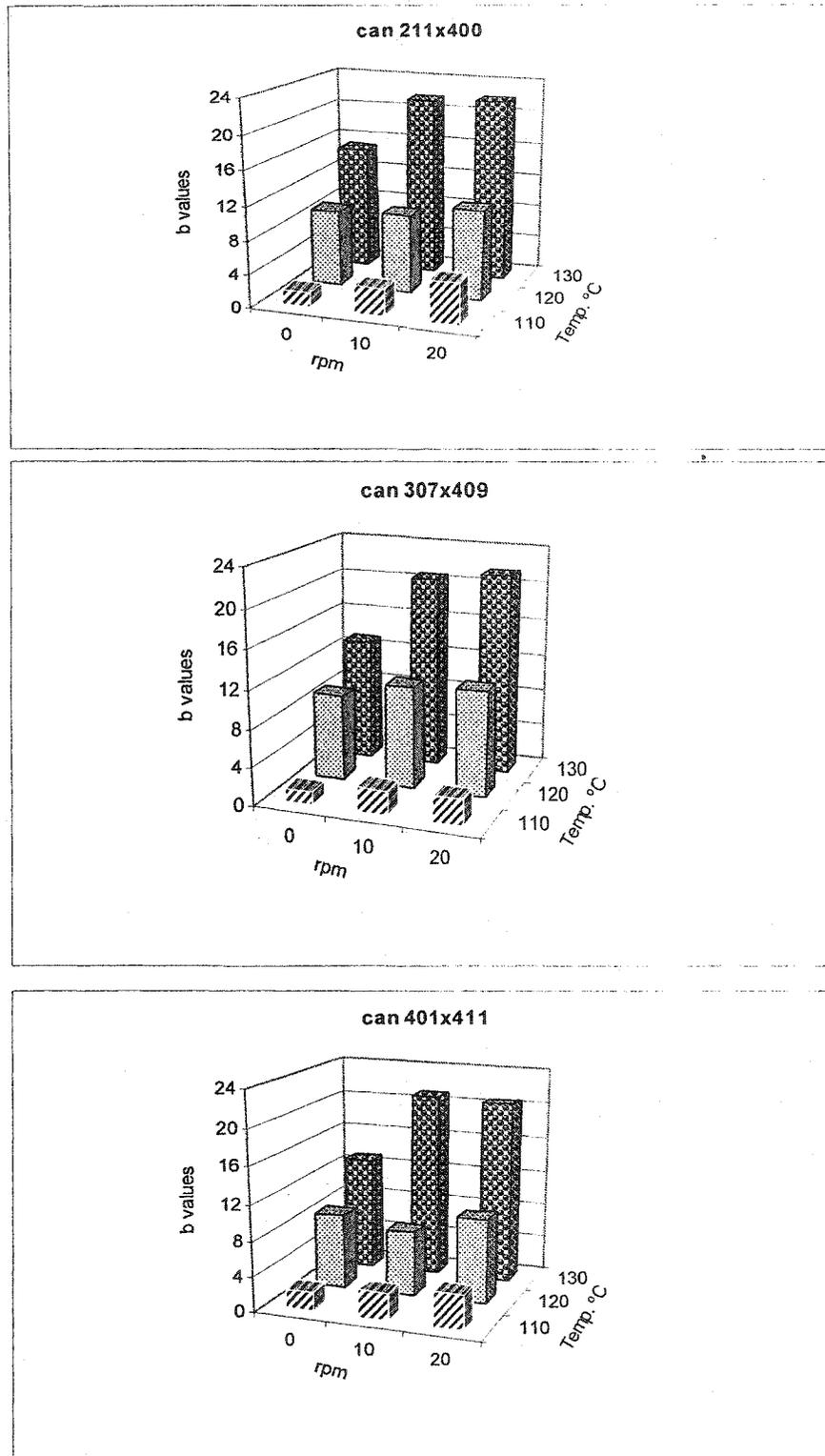
**Figure 5.6: Effects of temperature and rotational speed on b values of canned potatoes in CMC**
