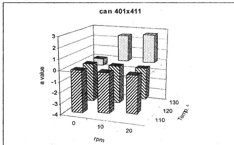
**Figure 5.4: Effects of temperature and rotational speed on 'a' values of canned potatoes in CMC**
