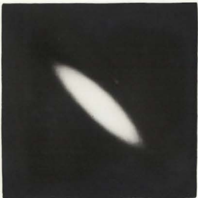
e) Correlation in an 800 cps band about 5000 cps Estimated Correlation, 60%
