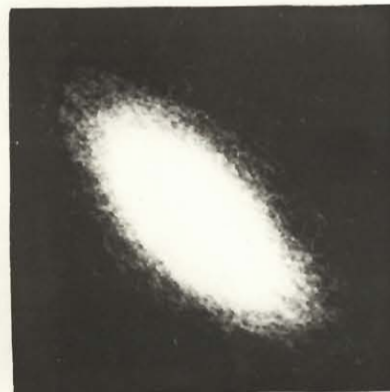
e) Correlation in a 35 cps band about 200 cps 10 second exposure Estimated Correlation, 50%
