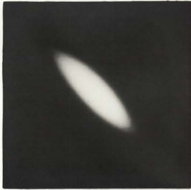
f) Correlation in a 1500 cps band about 10000 cps Estimated Correlation, 60%
