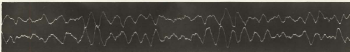
a) Correlated noise in a 4 cps band about 25 cps
