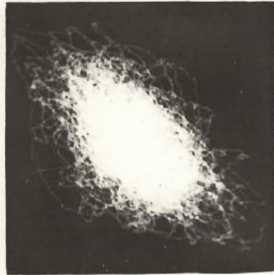
c) Correlation in a 4 cps band about 25 cps 10 second exposure Estimated Correlation, 40%
