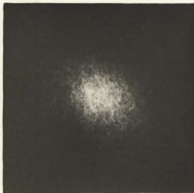
b) Correlation in a 120 cps band about 800 cps 1 second exposure Estimated Correlation, 15%
