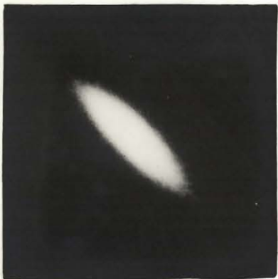
c) Correlation in a 200 cps band about 1250 cps Estimated Correlation, 60%
