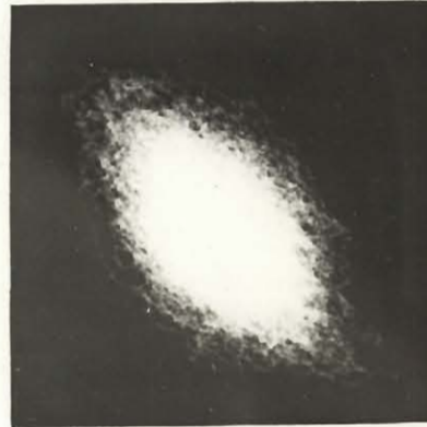
d) Correlation in a 12 cps band about 80 cps 10 second exposure Estimated Correlation, 40%
