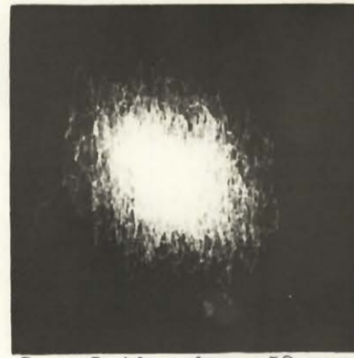
e) Correlation in a 50 cps band about 320 cps 1/2 second exposure Estimated Correlation, 25%
