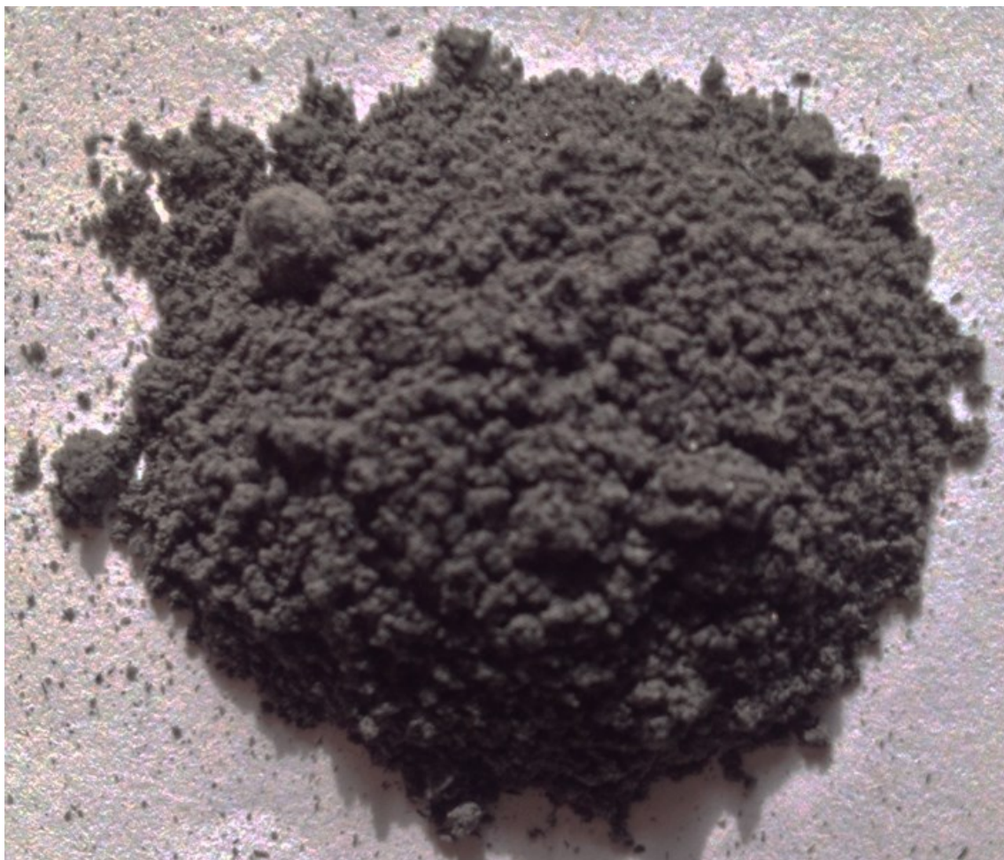
Figure S3- 3. Photo of the ground ash from switchgrass combustion. The mean particle size was 65.00 \mu\text{m} .
