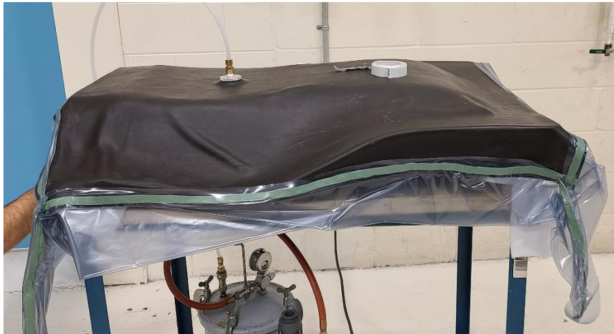
Figure 79 Vacuum bagging for rubber membrane preforming
