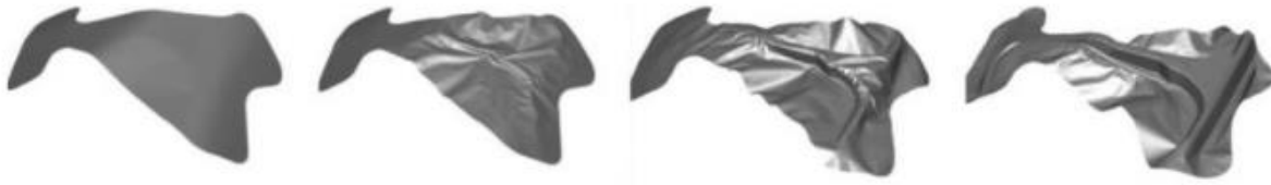
Figure 18 Example of preforming simulation using PAM-FORM (Copyright © ESI Group. All rights reserved [32])
