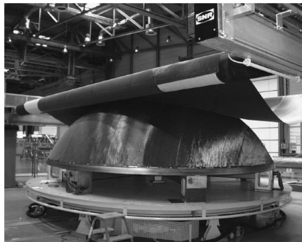
Figure 11 Use of NCF in aerospace industry: Draping of NCF in the Airbus A380 rear pressure bulkhead production (reproduced with permission from P. Middendorf [17])
