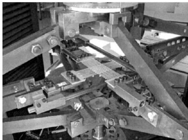
Figure 27 Biaxial tensile test device (reproduced with permission from Elsevier [54])
