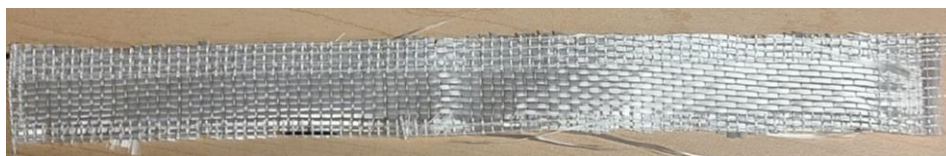
Figure 61 Dry-wall tape applied at the edge of fabric to reduce fraying
