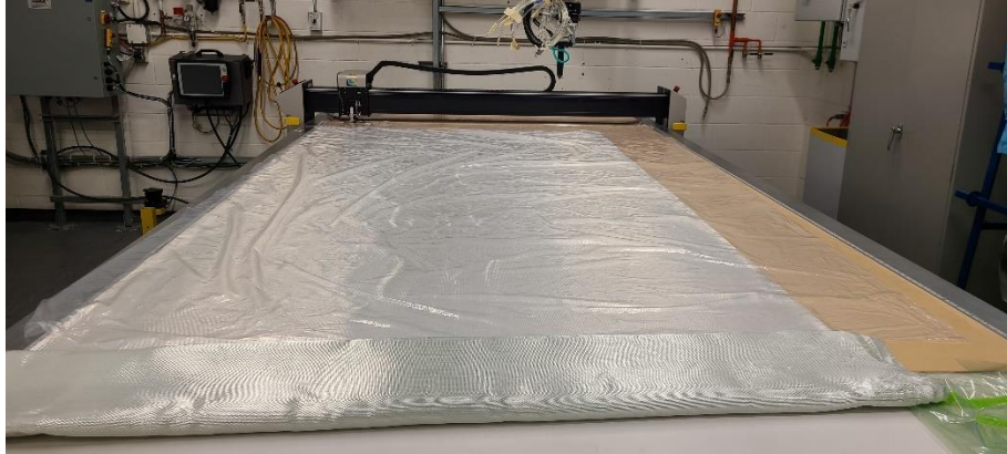
Figure 78 GERBERcutter® DCS 2500 Fabric cutting table at Centre Technologique en Aérospatiale (St-Hubert, QC)
